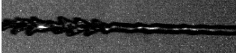
Figure 2.2: Wind induced breakup of a 50 \mu\text{m} liquid jet traveling from right to left with an average velocity 34.4 \text{ m s}^{-1} captured at 1Mfps.
