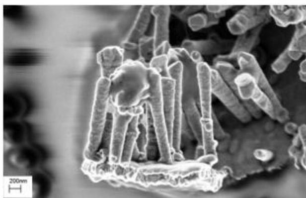
Figure 17: Result of the 200nm sputtered gold layer (after deposition and dissolution of the membrane)(HR)<sup>1</sup>.
