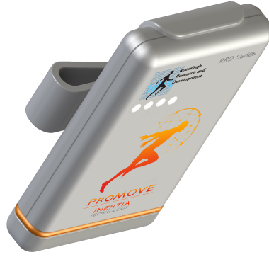
Figure 3.1: The ProMove3D sensor node, pictured with belt clip
