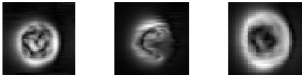
Figure 5.7: Some examples of the current in a ring when spontaneously generating a magnetic flux. The figures show high values of the current density |\mathbf{J}| in white while zero values of |\mathbf{J}| are shown as black. It can be seen that the currents are generally flowing on the edges of the ring as expected by the Meissner effect. Currents inside the ring are generally vortices. In these figures, the current circulates all the way around the ring.
