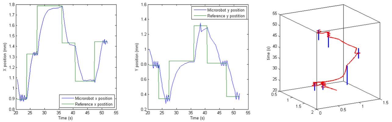
Fig. 11. Response of the diamond shaped  $50 \times 100 \mu\text{m}$  microrobot to closed-loop point-to-point control. In the first graph the x position of the microrobot is shown, in the second the y position and in the third a 3D-image of microrobot position in time.
