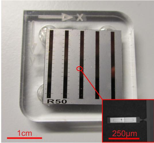
Fig. 2. A chip with 190 rectangular microrobots of width 50  $\mu\text{m}$  and lengths varying from 50 to 500  $\mu\text{m}$ . In the inset a magnification can be seen of one particular microrobot on the chip, as seen through the microscope.
