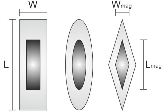
Fig. 3. Dimensions of the microrobots and the magnetic layers. W and L are the width and length of the microrobots whereas  $W_{\text{mag}}$  and  $L_{\text{mag}}$  are the width and length of the magnetic layer, respectively. These correspond with the values in table I.
