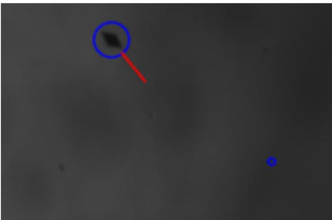
Fig. 7. This figure shows a snapshot of the closed-loop control of a diamond shaped microrobot of  $50 \times 100 \mu\text{m}$ . The large circle around the microrobot shows that it is being tracked. The line coming from the microrobot shows the velocity vector. The smaller circle shows the current reference point, to which the microrobot is moving.
