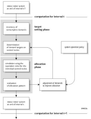
FIGURE 7: WORKING OF RIBASIM
