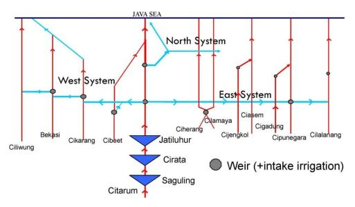
FIGURE 13: PJT II SCHEMATIZATION
