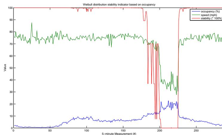
**Figure A.3** Stability indicator based on 8-days of historical data tested on data of April 4, 2013 on the I-880 Highway in California. Lane 2 of detector 400309 (Caltrans, 2013).
