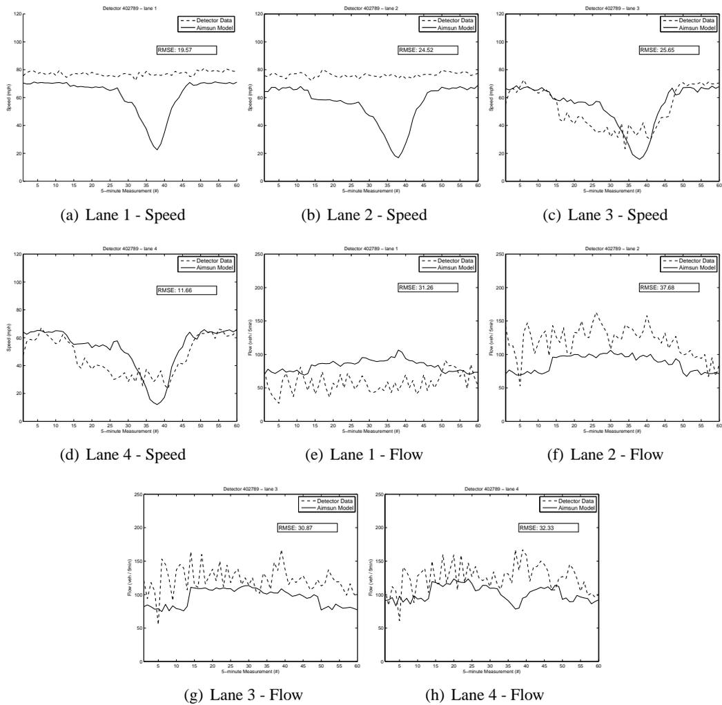
**Figure D.3** Calibration results of detector 402789 - post mile 12.4
