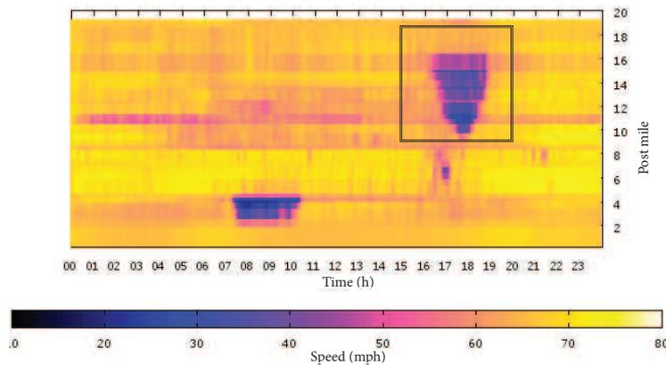
**Figure 6.1** The time-space speed contour plot for the I-880 NB on April 4, 2013 (Caltrans, 2013). Bordered is the considered section in the simulation model. The dark areas indicate low speed and can be determined as congestion areas.
