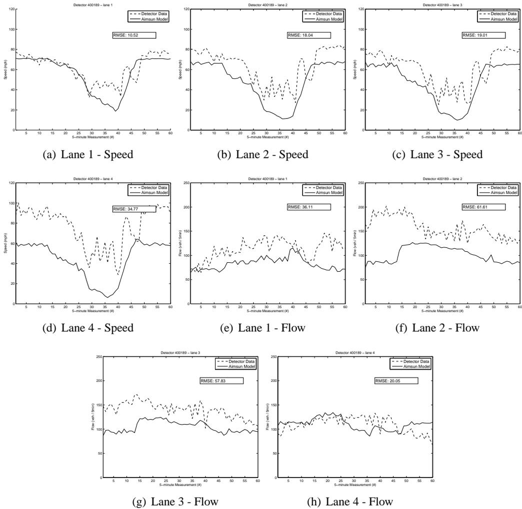
**Figure D.5** Calibration results of detector 400189 - post mile 13.51
