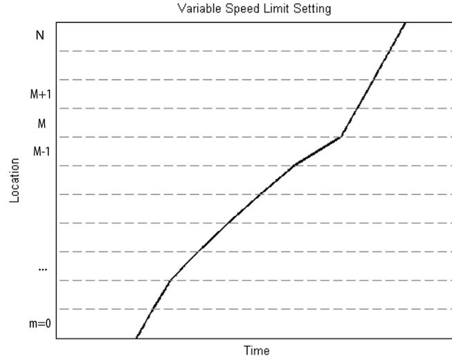
**Figure 5.2** Schematic visualization of the variable speed limit strategy where the speed limit in a link  $m$  is gradually decreased up to the bottleneck link  $M$ . Downstream links of the bottleneck, the most upstream link ( $m = 0$ ) and the bottleneck link itself, are not controlled.
