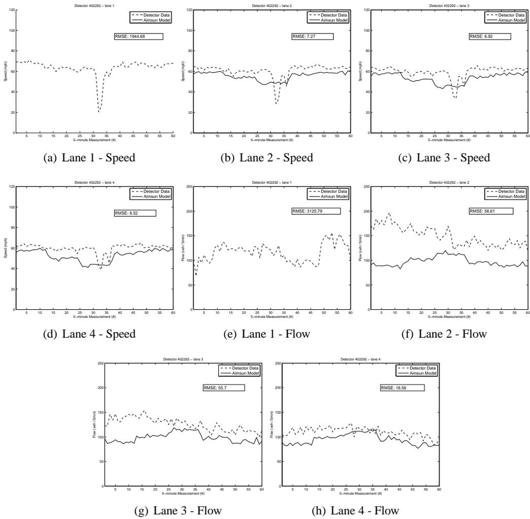
**Figure D.1** Calibration results of detector 402292 - post mile 9.80. Lane 1 has no model results due to technical issues.
