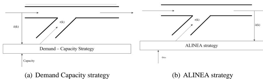
**Figure B.2** Schematic control of a local feed forward ramp metering strategy (a) and a local traffic responsive ramp metering strategy (after Papageorgiou et al. (1997)).
