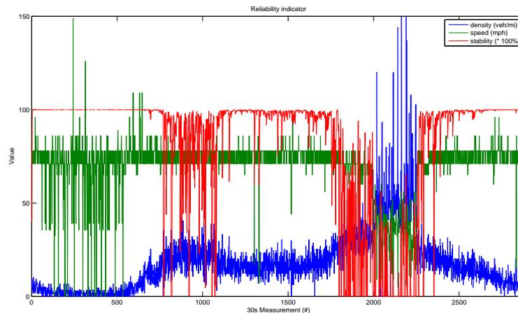
**Figure A.4** Reliability indicator based on 30s measurements data of April 4, 2013 on the I-880 Highway in California. Lane 2 of detector 400309 (Caltrans, 2013). Variance is based on the last 5 measurements.
