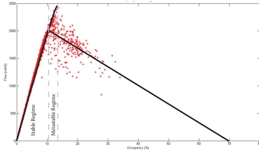
**Figure A.1** Schematic indication of metastable and stable regime based on 5-minutes occupancy-flow fundamental diagram. Notice the capacity drop and that the regimes are only indicated for free flow traffic.
