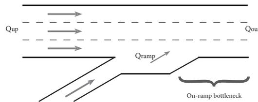
**Figure 3.1** Schematic indication of an on-ramp bottleneck. Three ingredients for congested traffic are available; high traffic volume ( $Q_{up} + Q_{ramp}$ ), a spatial inhomogeneity (merging lane drop) and perturbations caused by the merging vehicles.
