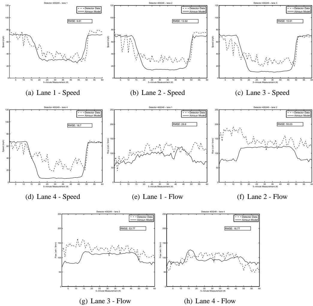
**Figure D.7** Calibration results of detector 400249 - post mile 14.89
