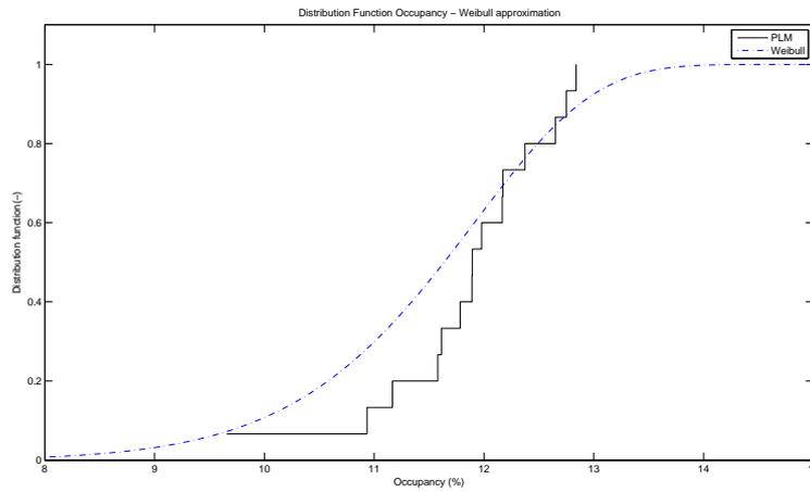
**Figure A.2** Product Limit Method and Weibull distribution function for breakdown, based on data of March 27, 2013 until April 3, 2013. Lane 2, detector 400309 (Caltrans, 2013).
