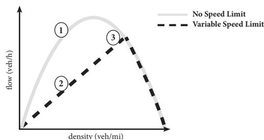
**Figure B.3** By setting a speed limit the (schematic) fundamental diagram changes from the gray to the dotted black line. Setting speed limits while traffic is in state 1, flow changes to somewhere between 2 and 3. Note that the speed limit should be lower than the static speed limit (after Hegyi et al. (2005)).
