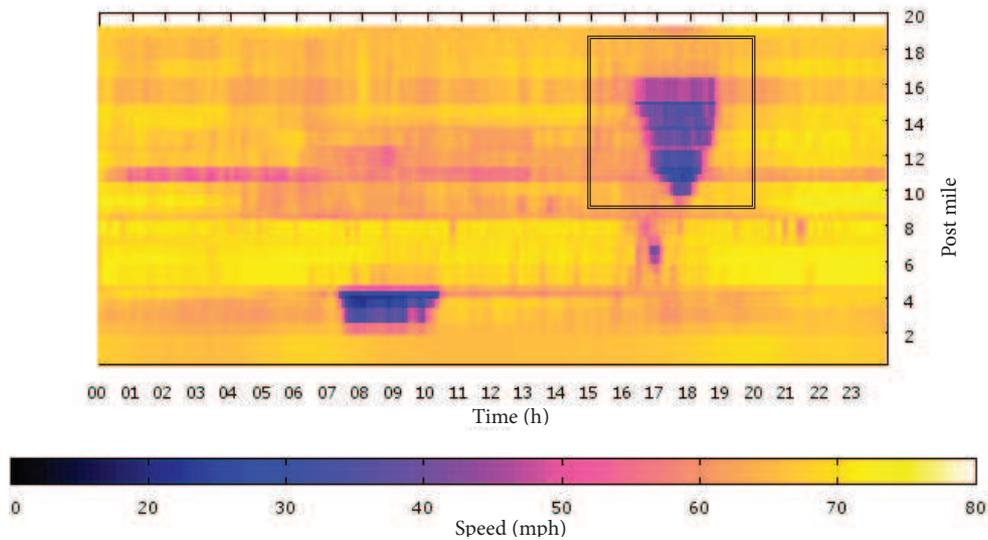
**Figure C.1** The time-space speed contour plot for the I-880 NB on April 4, 2013 (Caltrans, 2013). Bordered is the considered section in the simulation model. The dark areas indicate low speed and can be determined as congestion areas.
