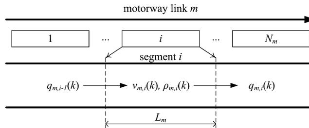
**Figure 5.4** The original METANET (Messner & Papageorgiou, 1990) discretized motorway link, after Kotsialos et al. (2002a).
