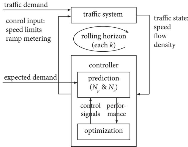
**Figure 5.3** Schematic Model Predictive Control scheme, after Hegyi et al. (2005)
