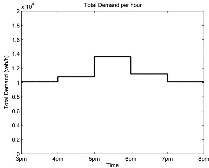
**Figure C.3** Demand per hour used for calibration of the simulation model. Total demand includes all inflow locations (on-ramps and mainline inflow) and all vehicle types.
