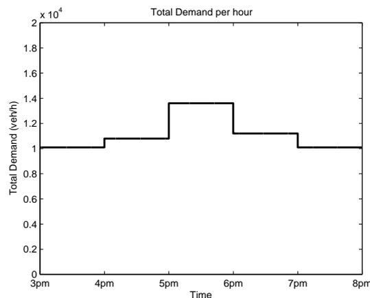
**Figure 6.2** Used demand in the simulation software. Demand includes all inflow locations (on-ramps and mainline) and all vehicle types.
