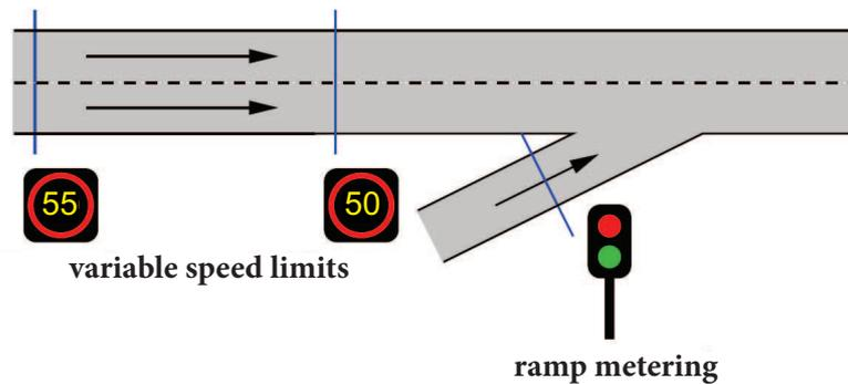
**Figure 4.1** Ramp metering and variable speed limits in order to control traffic (after Hegyi et al. (2005)).
