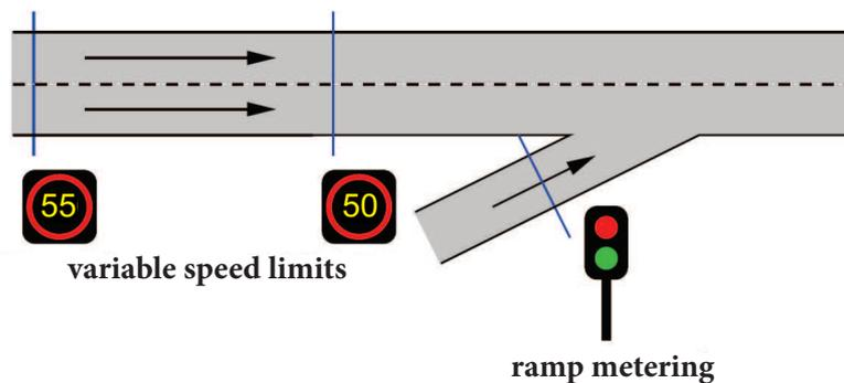
**Figure B.1** Ramp metering and variable speed limits in order to control traffic (after Hegyi et al. (2005)).
