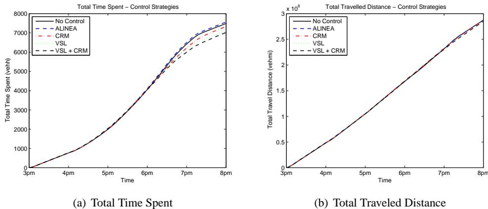
**Figure 6.3** Results of the microsimulation performance of the different control strategies. The integrated variable speed limit (VSL) and coordinated ramp metering (CRM) strategy is best performing. The local ramp metering strategy ALINEA does shows an increase in total time spent. The total traveled distance is not significantly changed due to different strategies.
