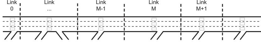
**Figure 5.1** Schematic corridor is divided into  $N$  links, every link with one set of detector and an on-ramp. The link where the congestion is detected is link  $M$ .
