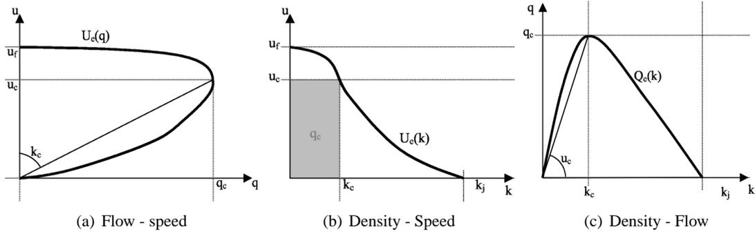
**Figure 3.2** Three related fundamental diagrams, assuming that traffic is stationary and homogeneous (Immers & Logghe, 2002).
