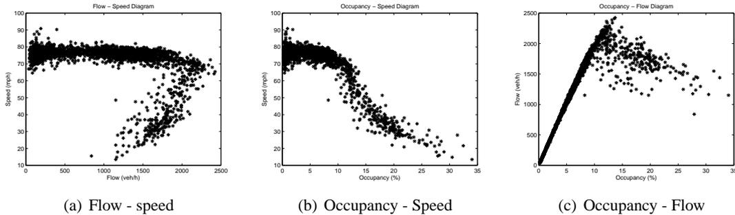
**Figure 3.3** Three related empirical fundamental diagrams, based on 5-minutes measurements of April 4, 2013 on the I-880 Highway in California. Lane 2 of detector 400309 (Caltrans, 2013).
