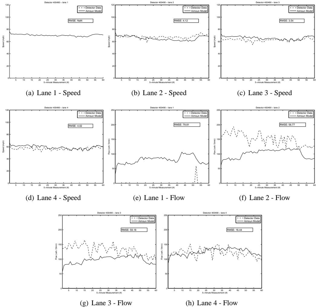
Figure D.11 Calibration results of detector 400490 - post mile 17.59
