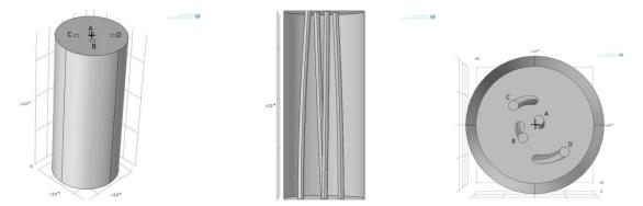
Figure 6: different views of the COMSOL model. Locations of the filaments from inside to outside, A to D.
