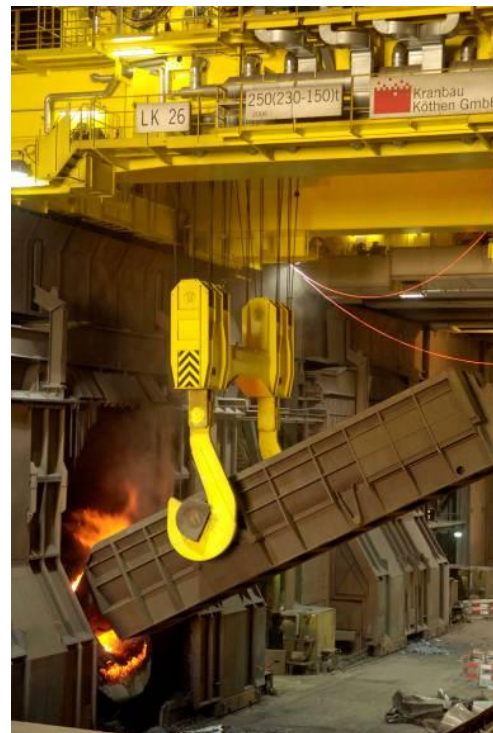
Figure 7 - Charging of scrap into a converter
