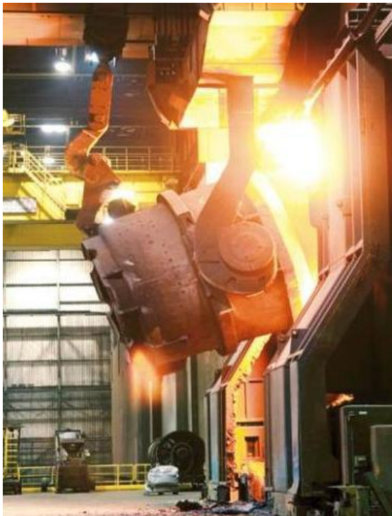
Figure 6 - Charging of pig iron into a converter
