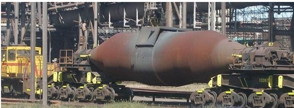
Figure 4 – hot metal car, transports the pig iron from the Blast-Furnaces to the Basic Oxygen Steel Plant (RolandRail.net, 2005)
