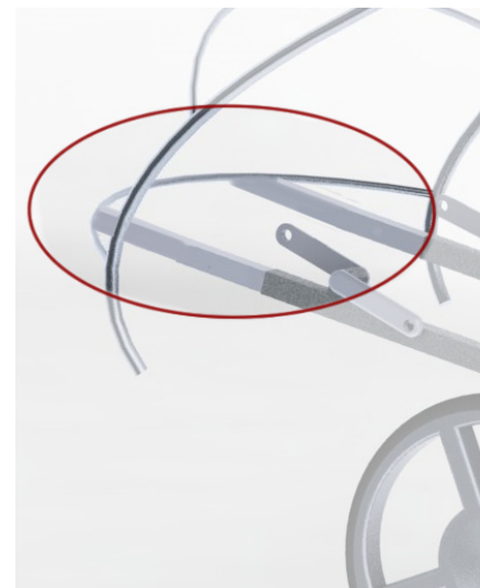
IMAGE 7.4: CONNECTION BETWEEN THE FRAME AND THE ROOF
