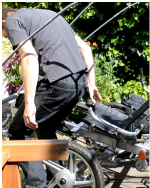
IMAGE 5.1: USER SITTING DOWN BY STEPPING OVER THE FRONT WHEEL
