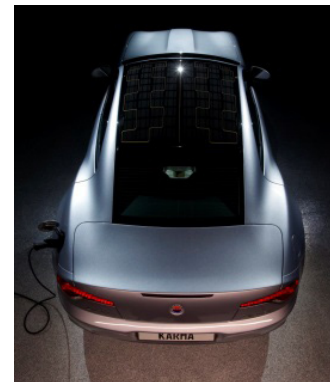
IMAGE 5.3: FLEXIBLE SOLAR PANEL ON A CAR [36]
