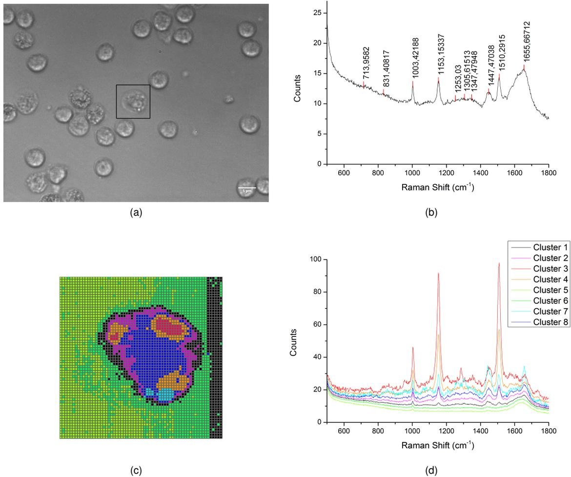
Figure 14: Measured lymphocyte with gall bodies on  $\text{CaF}_2$  with poly-L-lysine. (a) shows a white light image, (b) the average of 4096 spectra of a raster scan, (c) is a HCA image and (d) shows the corresponding HCA spectra. Raster scan ( $64 \times 64$  pixels) of  $6.4 \times 6.4 \mu\text{m}$ , 0.1s exposure time, readout rate 50kHz, gain 4x.
