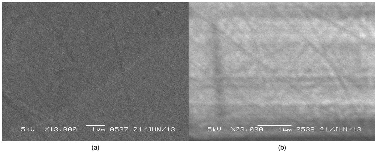
Figure 6: Surface of gold on  $\text{CaF}_2$  measured with SEM at a magnification of a) 13000x and b) 23000x using secondary electron imaging
