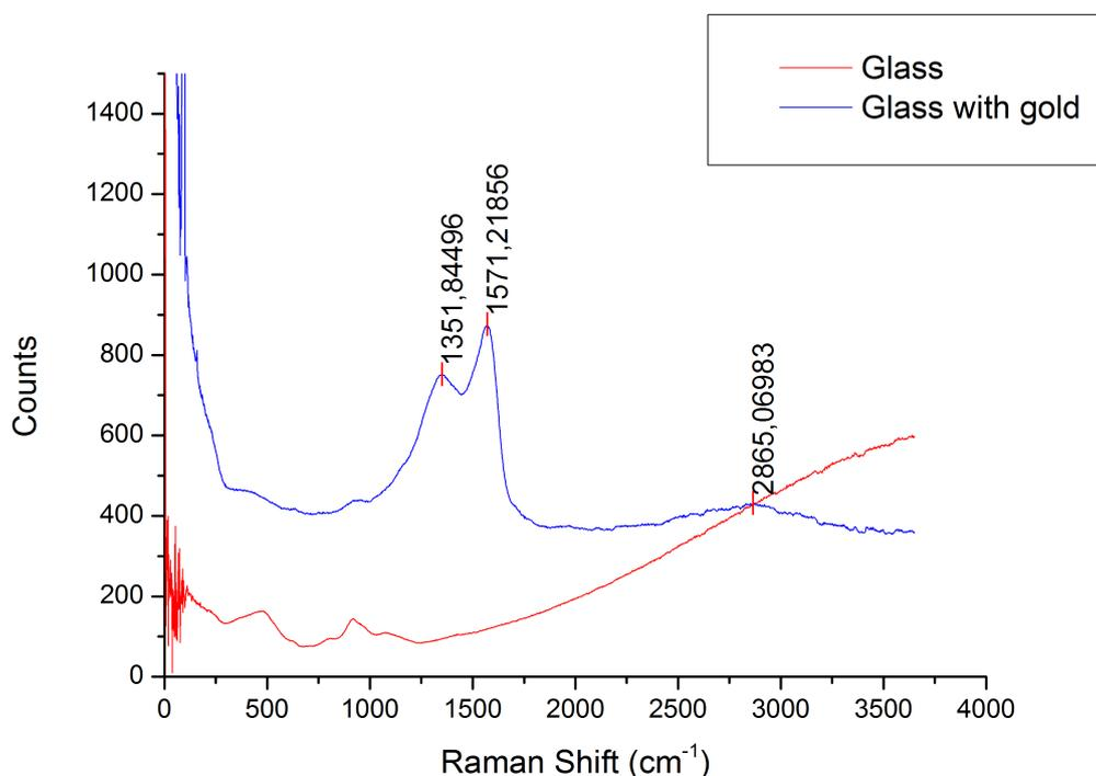
Figure 10: SERS effect on glass, average of 1024 spectra, 35mW laser power, 0.25s exposure time, readout rate 50kHz, gain 4x.
