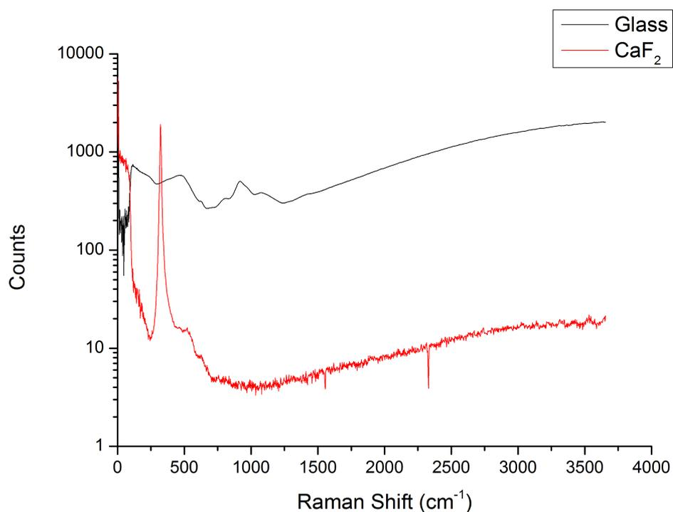
Figure 8: Raman spectra of expected background signal from  $\text{CaF}_2$  and glass, average of 1024 spectra, 35mW laser power, 0.25s exposure time, readout rate 50kHz, gain 4x.
