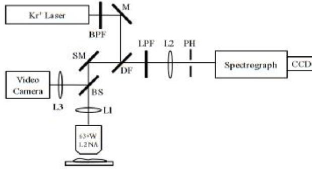
Figure 3: Schematic representation of Raman microscope. [13]
