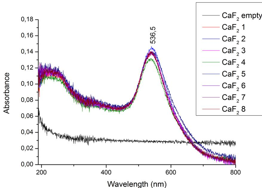
Figure 4: UV vis absorption of CaF<sub>2</sub> with air as reference and gold coated CaF<sub>2</sub> with empty CaF<sub>2</sub> as reference.
