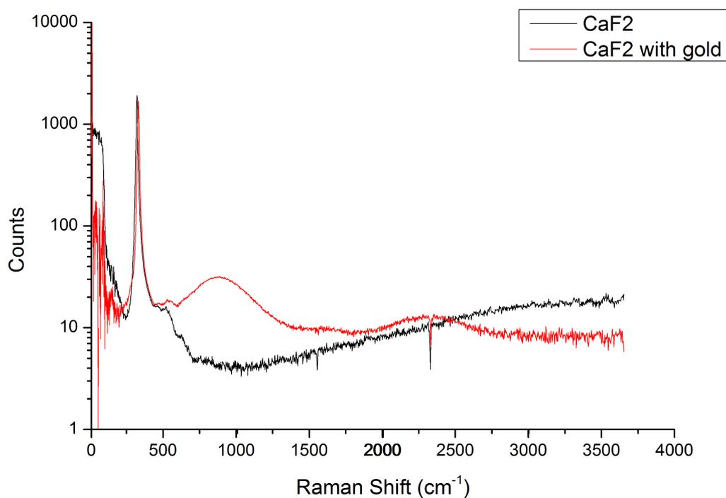
Figure 9: SERS effect on  $\text{CaF}_2$ , average of 1024 spectra, 35mW laser power, 0.25s exposure time, readout rate 50kHz, gain 4x.
