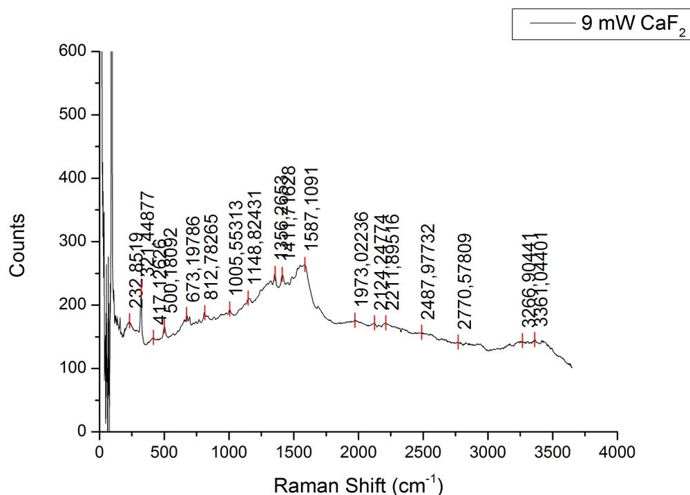
Figure 12: Peak analysis of Raman spectrum from opsonized gold coated CaF<sub>2</sub> at 9 mW laser power. Spectrum is average of 2048 spectra, 0.25s exposure time, readout rate 50kHz, gain 4x.
