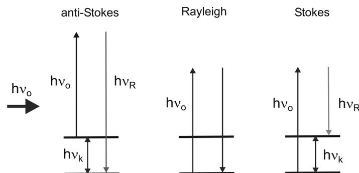
Figure 2: Molecular energy level diagrams illustrating light scattering. [4]
