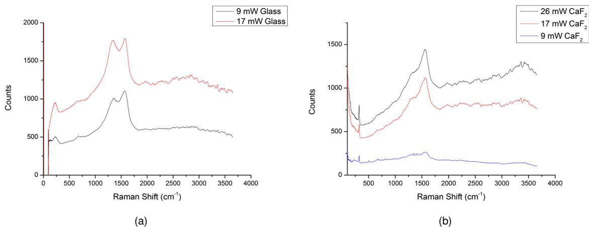
Figure 11: Raman spectra of opsonized, gold coated a) glass and b) CaF<sub>2</sub> substrates at different laser intensities. Spectra are average of 2048 spectra, 0.25s exposure time, readout rate 50kHz, gain 4x.
