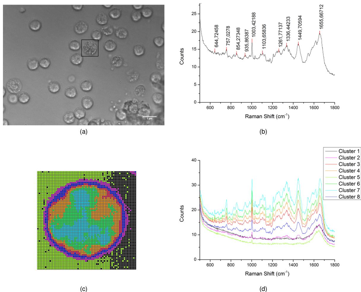
Figure 13: Measured lymphocyte on  $\text{CaF}_2$  with poly-L-lysine. (a) shows a white light image, (b) the average of 4096 spectra of a raster scan, (c) is a HCA image and (d) shows the corresponding HCA spectra. Raster scan ( $64 \times 64$  pixels) of  $6.4 \times 6.4 \mu\text{m}$ , 0.1s exposure time, readout rate 50kHz, gain 4x.
