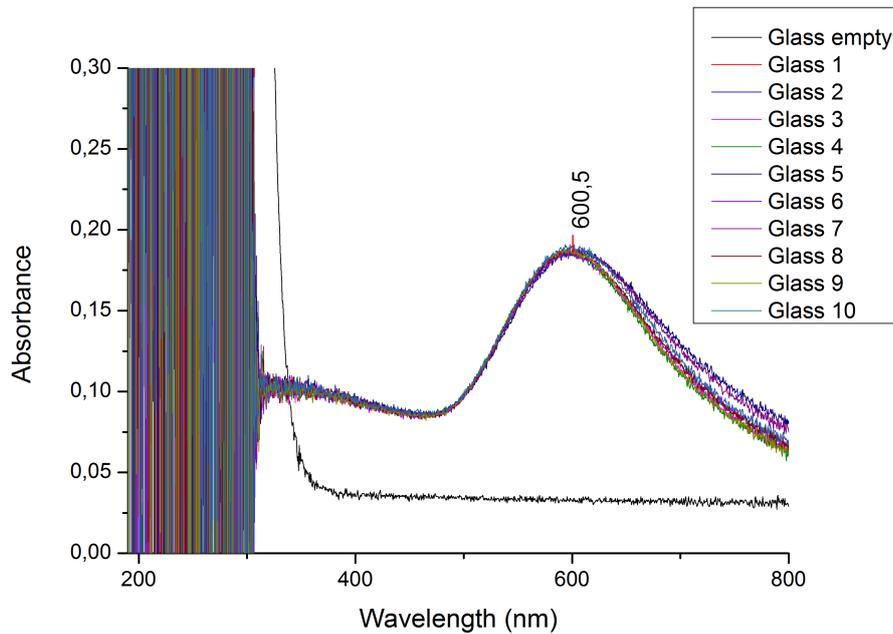
Figure 5: UV vis absorption of empty glass with air as reference and gold coated glass with empty glass as reference
