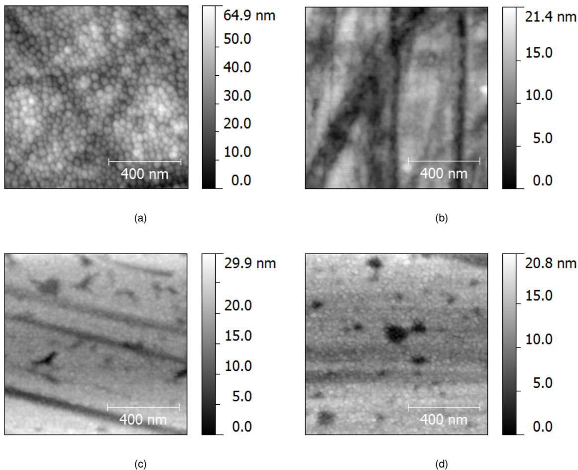
Figure 7: AFM images from (a)  $\text{CaF}_2$  with gold, (b)  $\text{CaF}_2$  without gold, (c) glass with gold and (d) glass without gold.
