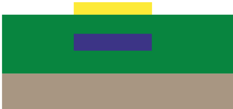
Figure 1.3: Cross-sectional schematic of part of a ring with a heater on top. The grey area is the silicon wafer. The cladding layers of \text{SiO}_3 are green. The \text{Si}_3\text{N}_4 core is blue. The yellow part on top is the gold heater.
