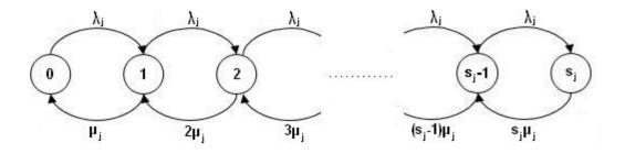
This is the well-known M/M/s/s queue, which is generally used to describe a queue with exponential inter-arrival and repair times and a finite (s-sized) number of servers. This system is also known as the Erlang Loss Model. The steady state probabilities for this model are relatively easy to determine, and are given by
