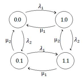
Here the first number denotes the number of broken items of type one, and the second number denotes the number of broken items of type two. Note that this system has only one operating state, namely the (0,0) state. If one of the two items is broken the system can be considered unoperational.
