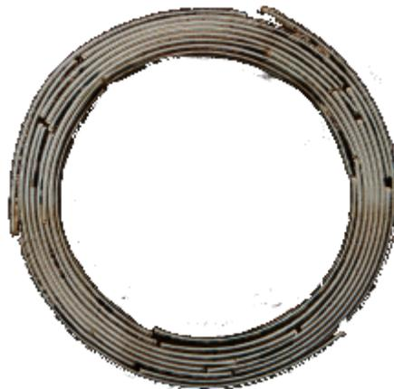
Figure 2.1: Cross section of a YBCO CORC cable. The stainless steel core around which the YBCO is wound is not displayed.
