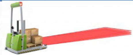
Figure 1.29: Laser target navigation
