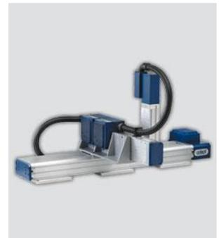
The Adept Python linear module's 'reach' varies between 100 mm and 2000 mm, depending on the requirements. Supporting a maximum payload of 160 kilograms, it is able to reach speeds up to 1450 mm per second. Due to the static nature of Cartesian robots, this type of robotics is not considered efficient to account for in the design.
