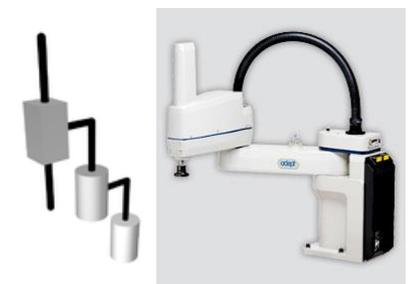
Cobra SCARA robots possess a higher level of accuracy compared to the standard 6 axis robots, with an XY plane repeatability of 0.017 mm and 0.003 mm in the Z axis (Adept Technologies, 2013). Specifications of this product indicate joint speeds between 386 and 1200 degrees per second, thus allowing for faster execution of tasks compared to the 6 axis robots.
