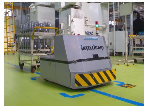
Figure 1.30: Magnetic tape navigation
