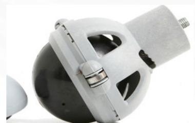
Figure 1.10: spherical wheel
