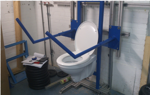
11.7 - Prototype hangend in de testopstelling
