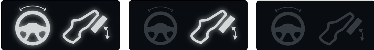
Fig. 7.16, 7.17 and 7.18: The human status indicators in Inform state (in both directions), lateral Assist plus longitudinal Inform state and complete take over state. The steering wheel represents the steering task and the pedal the task of handling the gas and brake pedal.
