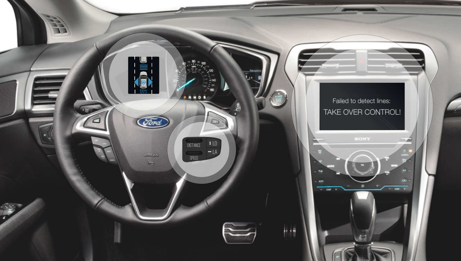
Fig. 7.1: Placement of the interface in the vehicle. The main system status is shown in the cluster display, 'feed afters' in the middle console display and controls are placed at the steering wheel.
