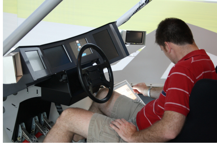
Fig. 8.5: During the experiment the interface is shown at the dashboard (behind the steering wheel). The middle console is used by the participant to perform a secondary task.
