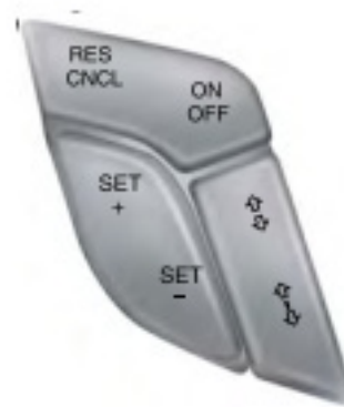
Fig. 2.3 The controls of ACC which are placed at the steering wheel.
