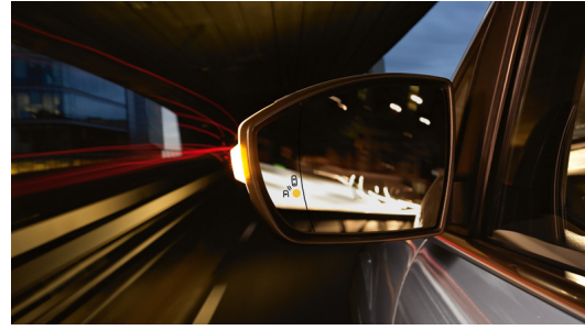
Fig. 2.7 The indicator light of BLIS, implemented in the side mirror.
