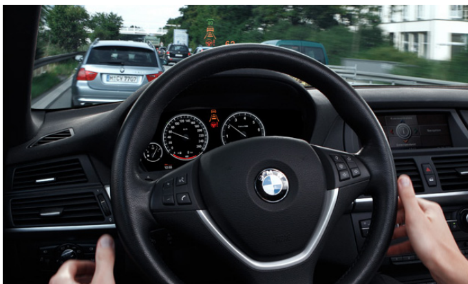
Fig. 2.14. BMW's TJQA, displayed at both the cluster and a Heads Up Display during automated driving.
