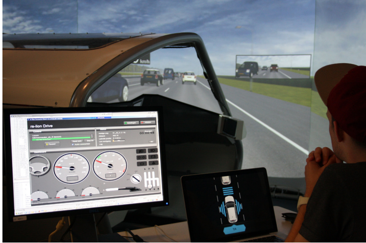
Fig. 8.4: During the experiment the interface and simulator are constantly monitored. Steering wheel and pedal activity is measured as well as reaction times.
