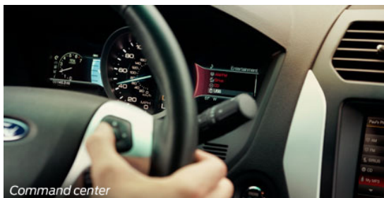
Fig. 2.8 The command center, from which SYNC is controlled with steering wheel buttons, in the cluster display.
