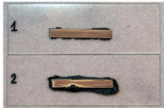
The silver layer is etched by solution of hydrogen peroxide 35% with water and ammonia. The ratio is 1:1:1. It's better to add a cold water to hydrogen peroxide and then add ammonia, because mixing hydrogen peroxide with ammonia leads to self-heating process.
