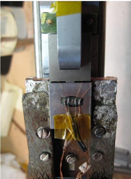
Sample soldered to current leads and voltage tabs connected
