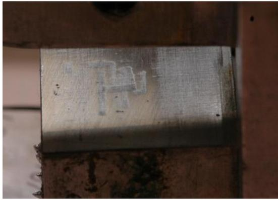
IMAGE 3-2: ANVIL AFTER SHORT POLISHING, DAMAGE IS CLEARLY VISABLE
