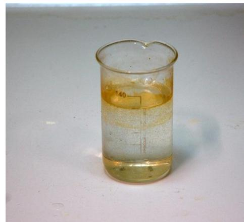
After silver etching samples needed to be extensively flushed with water to remove residual etching chemicals.
