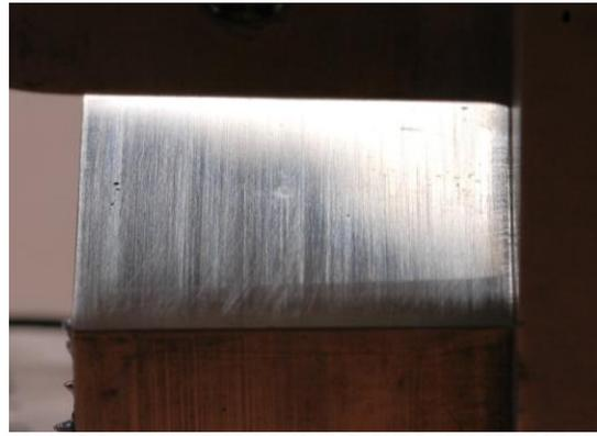
IMAGE 3-3: ANVIL AFTER POLISHING, THE DAMAGE HAS BEEN REMOVED
