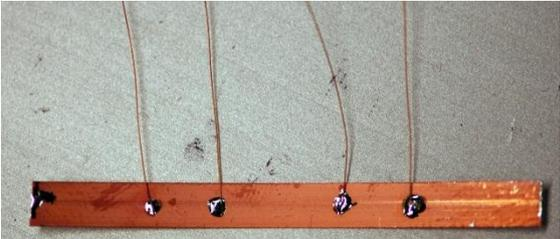
Voltage tabs connected to sample as described in step 14.
