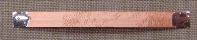
Pre-tinned side of sample that will be connected to current leads as described in step 15.
