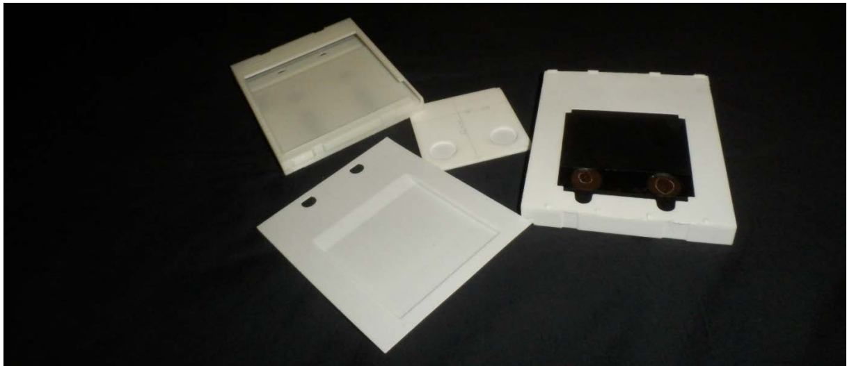
FIGURE 48 PROTOTYPES MADE USING 3D PRINTING
