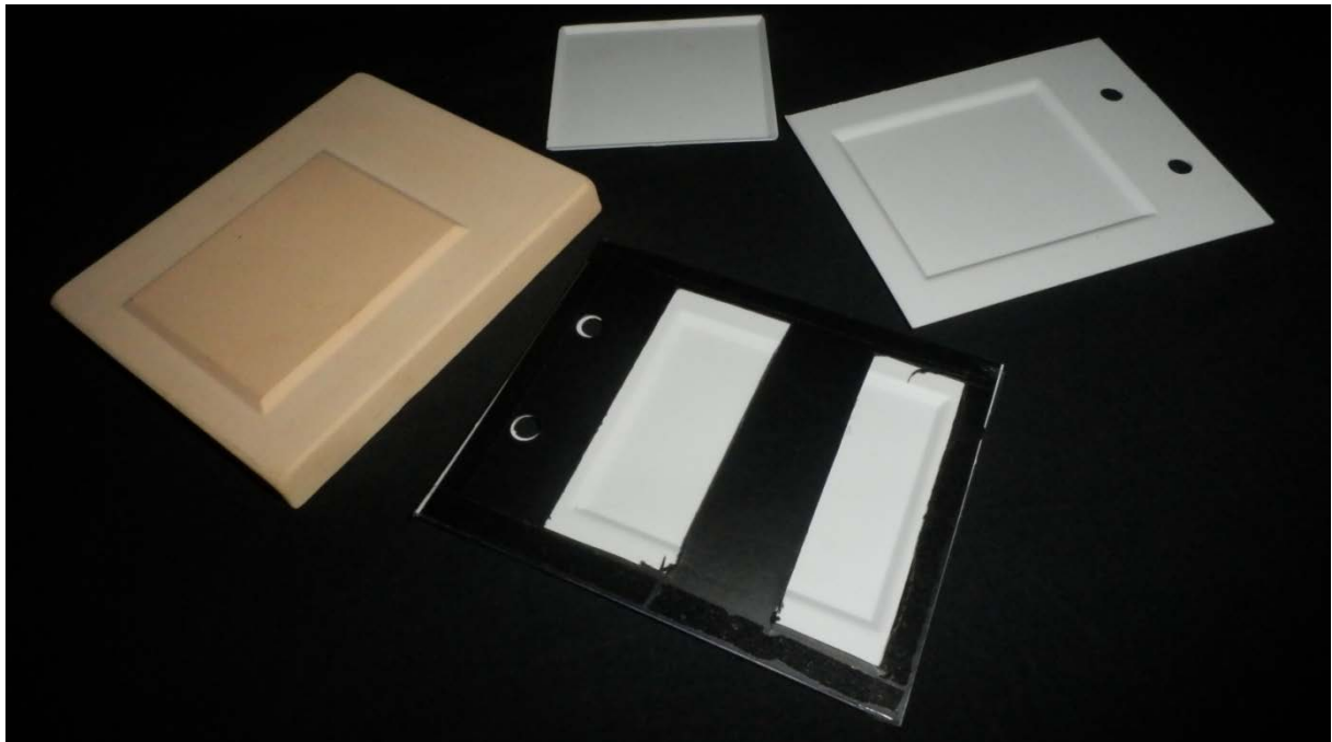
FIGURE 46 PROTOTYPES MADE USING VACUUM FORMING
