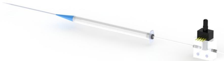
**Figure 3.12** – Representation of the syringe, capillary and pressure sensor free from the setup. The filter is placed in front of the pressure sensor in order the measure the actual pressure applied to the capillary.
