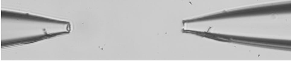
**Figure 3.9** – A  $10\mu\text{m}$  capillary 10x magnified. It can be observed that the mirrored capillary on the left is slightly rotated with respect to the capillary on the right. Note that this may seem like a huge rotation, but the capillaries are made of glass so they are translucent. This makes it hard to see the actual opening. In addition, the mirrored capillary has been rotated in both  $\theta$  and  $\phi$  direction.
