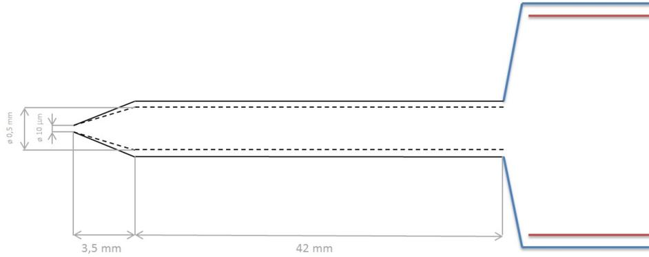
**Figure 3.14** – For the  $1\mu\text{m}$  and  $100\text{ nm}$  capillaries the inner diameter of course reads respectively  $1\mu\text{m}$  and  $100\text{ nm}$  and not  $10\mu\text{m}$ . The inner diameter is represented by the dashed black line. The Luer lock is indicated by the thick blue lines and the syringe by the red lines. So the parts that play a role in the time of the filling process are black in this figure.
