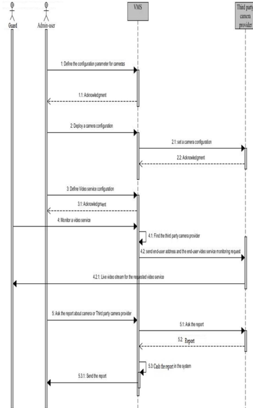
Figure 4.3 Interactions with external entities to provide a Video monitoring application
