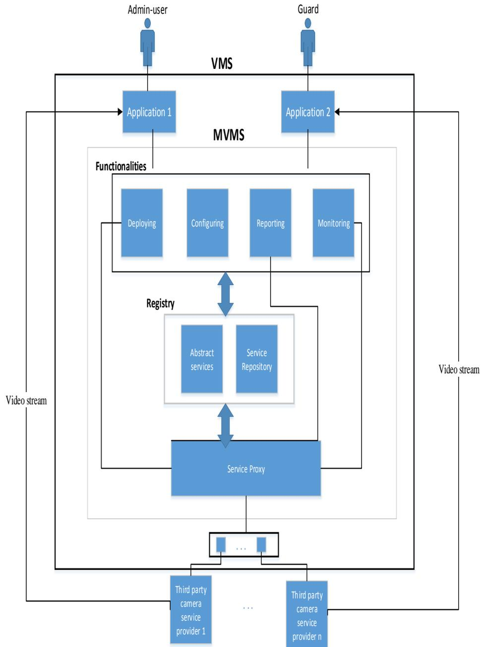
Figure 5.3 Overview of the VMS system including the applications and MVMS
