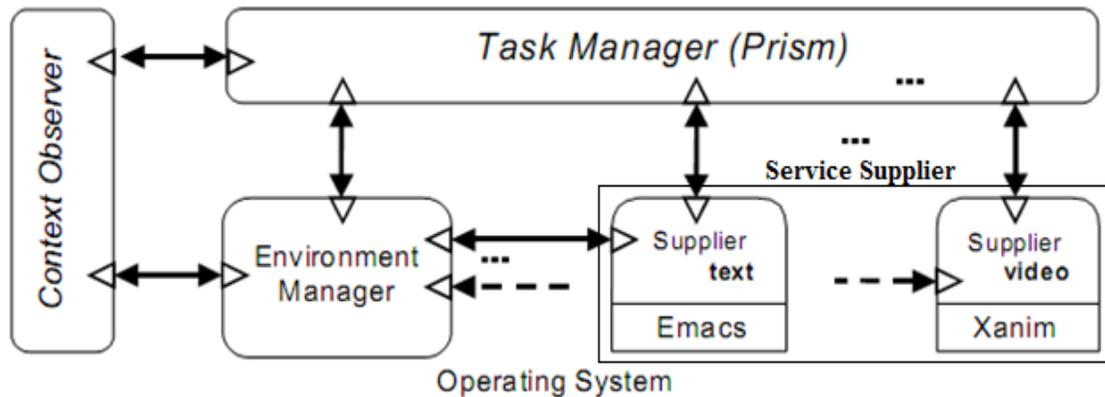
Figure 3.1 The components of the AURA framework architecture and their interactions.
