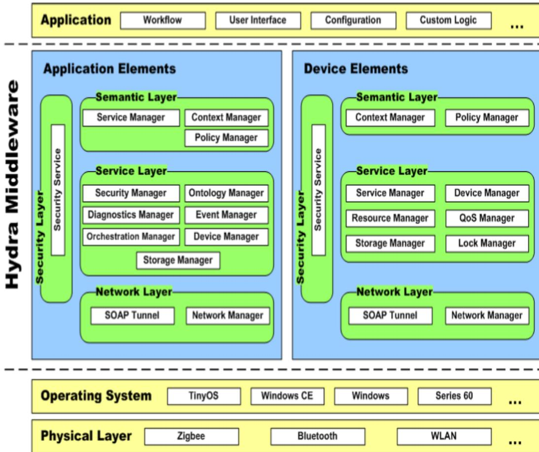
Figure 3.2 Components inside and outside of Hydra middleware.
