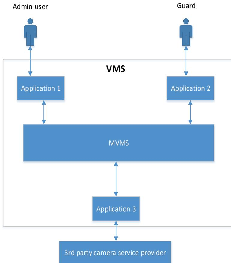
Figure 4.1 High-level architecture of a VMS
