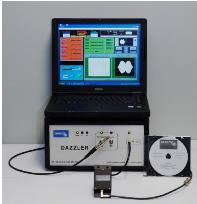
Figure 4.2: The complete Dazzler system consisting of the RF driver, the crystal module and a dedicated computer running the Dazzler software.
