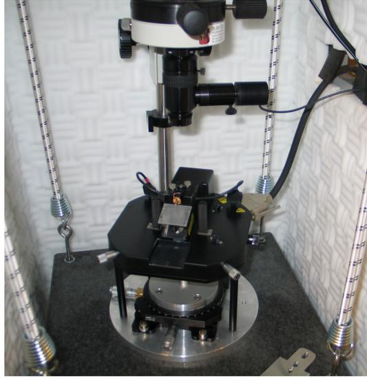
Figure 12: Agilent 5100 Atomic Force Microscope.
