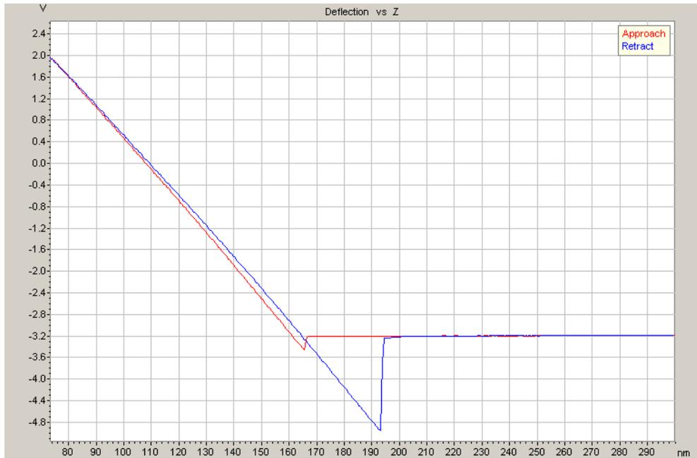
**Figure 17: Force distance spectroscopy measurement on a CrN sample. The x axis measures the tip position and the y axis the voltage value that the photodetector creates.**
