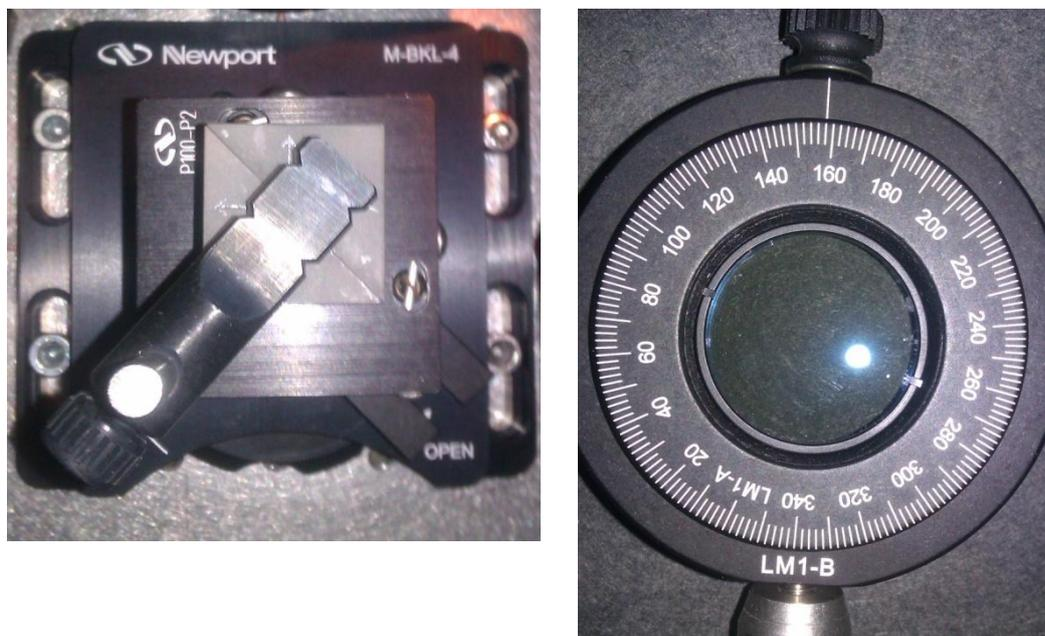
**figure 5.2: Photograph of the polarizing beam splitter (left) and the polarizer, placed in the rotation mount (right)**
