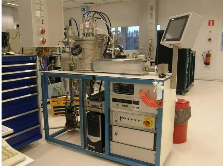
**Figure 3.4** – One of the magnetron sputtering systems available in the MESA+ cleanroom. This particular system is nicknamed "Sputterke". Photo by MESA+ cleanroom staff.
