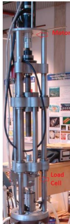
Figure 12: Motor stage.
