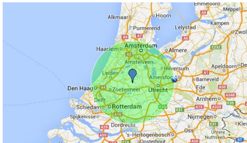
Figure 4.13: graphical representation of the 100% successful coverage area (arrival time \leq 10 minutes) of a helicopter flying between Rotterdam and Amsterdam.
