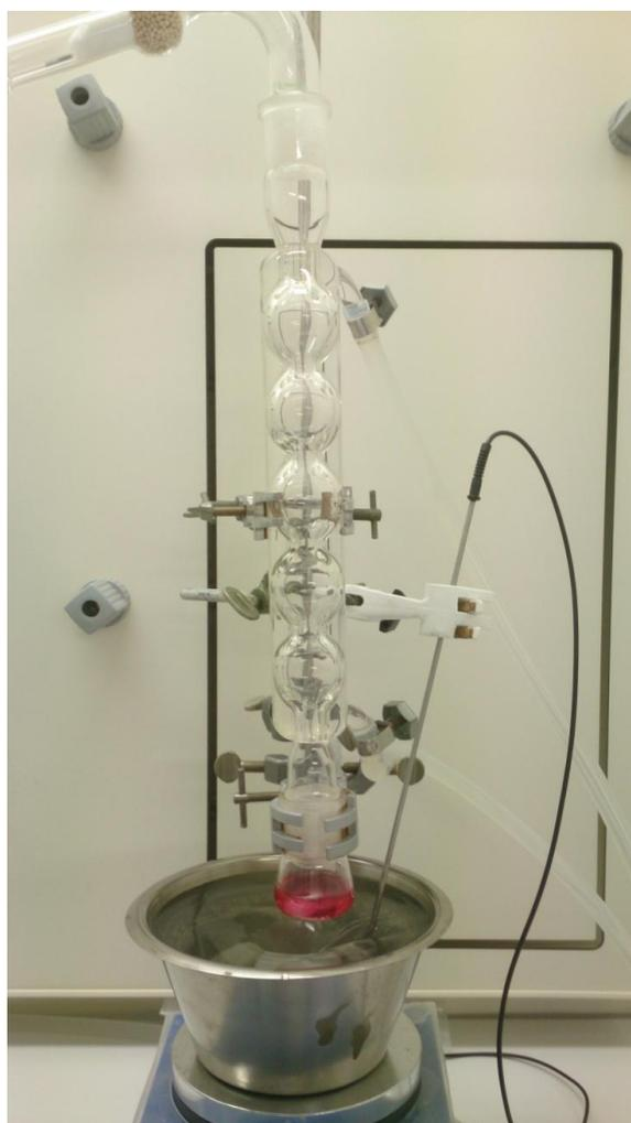
**Figure 7: The set-up used for the synthesis cobalt-doped sols**
