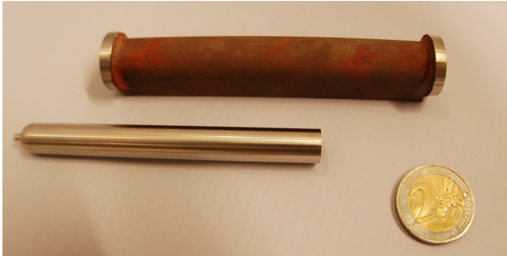
Figure 4.3: A photograph of the carbon inside a container and the corresponding heat sink.
