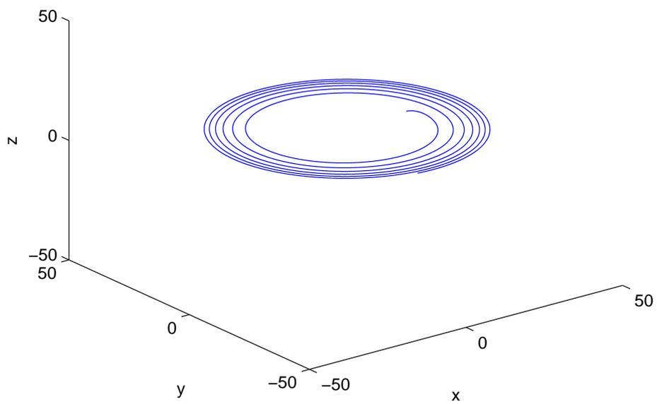
Figure 2.9.: The roost attraction causes the bird to turn its forward direction 'perpendicular' to the roost and spiral toward the steady state radius. In this experiment, the bird started of in  $(20, 1, 10)^T$  with velocity  $(10, 0, 0)^T$  and level flight.
