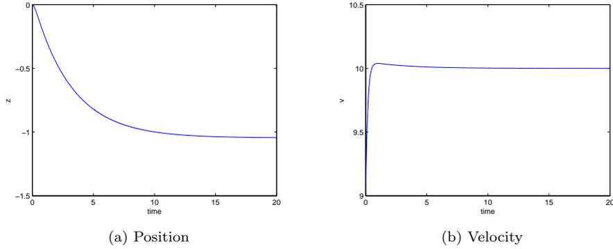
Figure 2.4.: When the bird has an initial velocity that is lower than the cruising speed, gravitational will be stronger than the lift and the bird will descend. The thrust will exceed the drag, so the bird will gain speed. The initial state is  $\mathbf{v} = (v_0 - 1, 0, 0)^T$ ,  $\mathbf{p} = (0, 0, 0)^T$  and  $\beta = 0$ , and  $v_0$  is  $10 \text{ ms}^{-1}$ .
