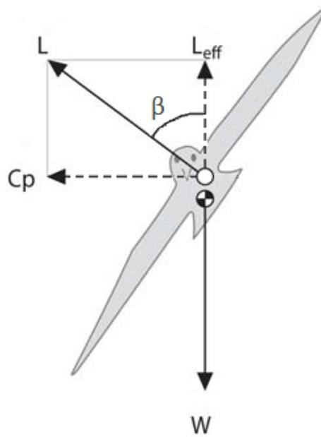
Figure 2.6.: If the banking angle  $\beta$  is not equal to zero, the lift has a horizontal component  $C_p$  that works as a centripetal force and pulls the bird into a circular path.[7]
