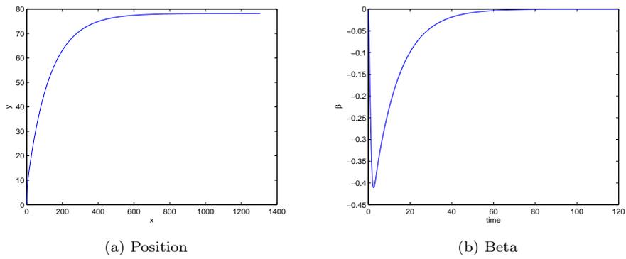
Figure 3.2.: The response to a constant force in the positive  $x$  direction. The initial state for the bird is given as  $\mathbf{v} = (0, v_0, 0)^T$ ,  $\mathbf{p} = (0, 0, 10)^T$ ,  $\beta = 0$  and  $\omega = 0$ .
