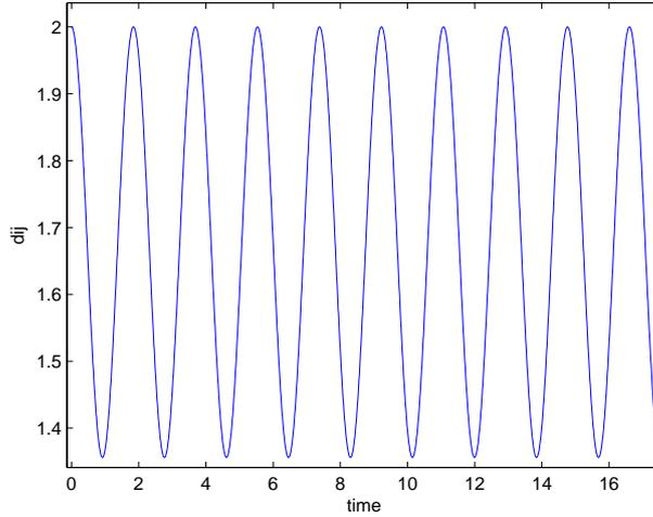
Figure 2.13.: The separation and cohesion force produce an oscillating solution. That is the result of the near linear behavior of the separation force around the equilibrium point. In this experiment, two birds were started  $2m$  apart on the x-axis, with their directions along the x-axis.
