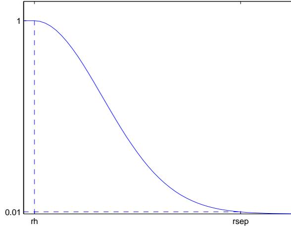
Figure 2.10.: The weighting factor  $g(d_{ij})$ , given in Equation (2.24b) determines how strongly a bird reacts to his neighbors. It is modeled so that it is almost zero at the edge of the separation zone  $r_{sep}$ . If the distance is smaller than  $r_h$ , there is no cohesion and birds repel each other.
