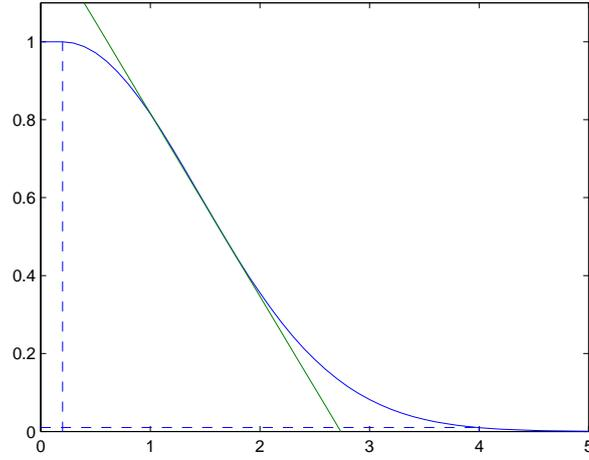
Figure 2.12.: The linear approximation of  $g(d_{ij})$ [The linear approximation of  $g(d_{ij})$  around the equilibrium position. It shows that for small deflections, the linear approximation of the separation force suffices to find the behavior induced by separation and cohesion that is shown in Figure 2.13
