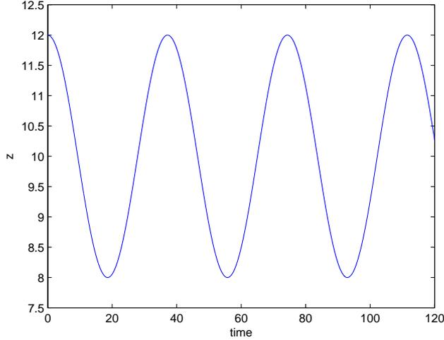
Figure 2.8.: When only altitude control is applied, the solution to the system will oscillate around the zero level. Here, the initial state of the system is given by  $\mathbf{v} = (v_0, 0, 0)^T$ ,  $\mathbf{p} = (0, 0, z_0 + 2)^T$  and  $\beta = 0$
