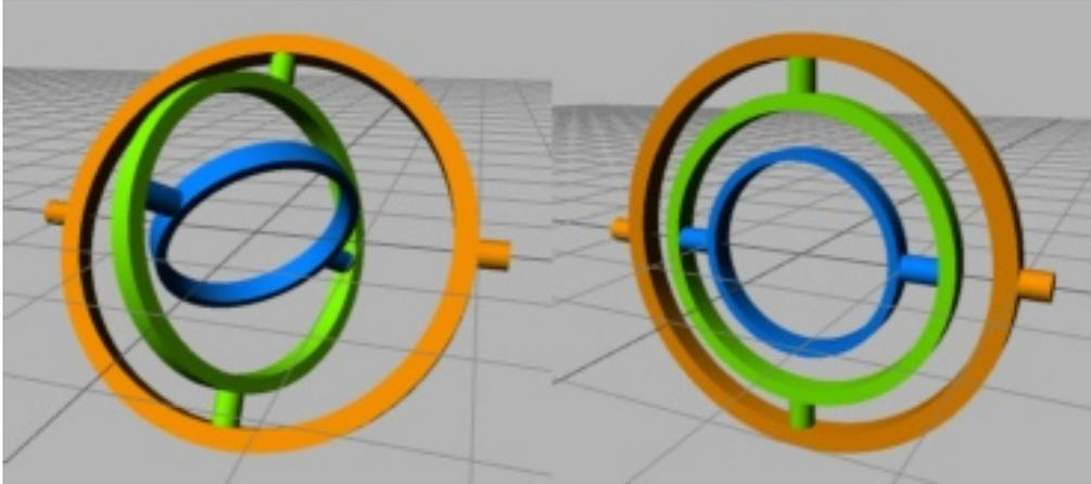
Figure 3.1.: The Tait-Bryan angles are illustrated using gyroscopes, consisting of three gimbals. The orange gimbal represents the heading, green the elevation and blue the banking. When the three rings align, as they do on the right, the system is locked in two dimensional rotation.[16]
