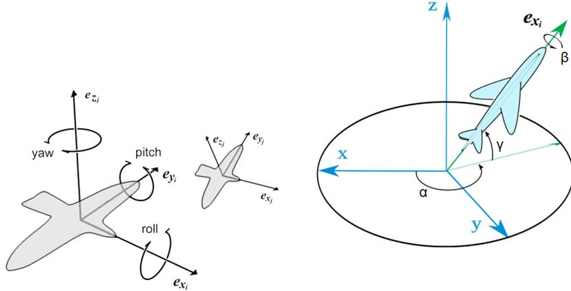
(a) The local coordinate systems of two birds,  $i$  and  $j$ . The forward direction for an individual  $i$  is called  $\mathbf{e}_{x_i}$ ,  $\mathbf{e}_{y_i}$  is the lateral direction and  $\mathbf{e}_{z_i}$  is the upward direction. Rotation around  $\mathbf{e}_z$  is called yaw, rotation around  $\mathbf{e}_y$  is called pitch and rotation around  $\mathbf{e}_x$  it is called roll.[8]
