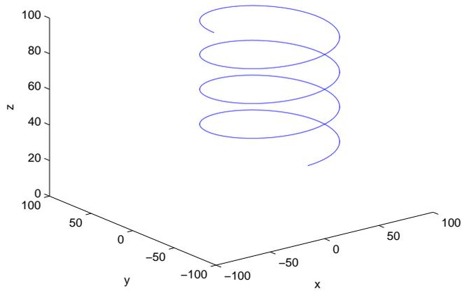
Figure 2.5.: If the banking angle is constant, there will be a constant centripetal force and the bird will fly in a circle. Since the effective lift is lower than the weight, the bird will also drop. The initial state  $\mathbf{v} = (0, 2v_0, 0)^T$ ,  $\mathbf{p} = (-25, 0, 100)^T$  and  $\beta = 0.2$  results in a downward helix, as predicted.
