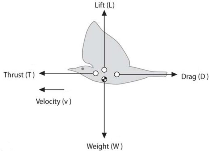
Figure 2.2.: The flight force  $\mathbf{F}_{\text{Flight}}$  consists of four elements: lift, drag, thrust and weight. The lift is directed towards the local upwards direction  $e_z$  and gravity towards the global downwards direction. Thrust points in the forward direction  $e_x$  and is opposed by the drag force.[7]
