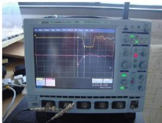
Figure 3.2: A cosmic ray traversed the scintillator and the spark chamber.
