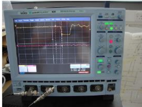
Figure 3.1: The yellow (top) line represent the signal from the coincidence module of the spark chamber. The pink (bottom) line represents the signal from the scintillator. A cosmic ray particle traversed the spark chamber but not the scintillator.
