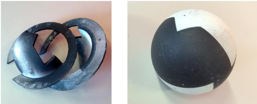
Figure 3.2: A finished painting stencil after several uses (left) and an example sphere as spray-painted using the stencil (right).
