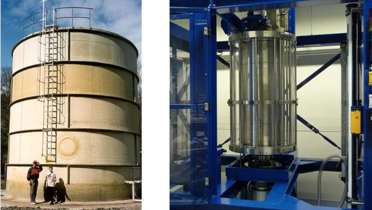
Figure 5.5: Barrel of Ilmenau (left), courtesy of Technische Universitaet Ilmenau, Institute of Thermodynamics and Fluid Mechanics and the Twente Turbulent Taylor-Couette system (right), courtesy of the Physics of Fluids Group, University of Twente
