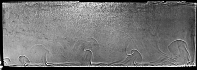
Figure 6.14: Shadowgram as created by the setup. It is difficult to capture the perception as viewed by the naked eye on paper, though this contrast-adjusted image shows good resemblance with the actual shadowgram.
