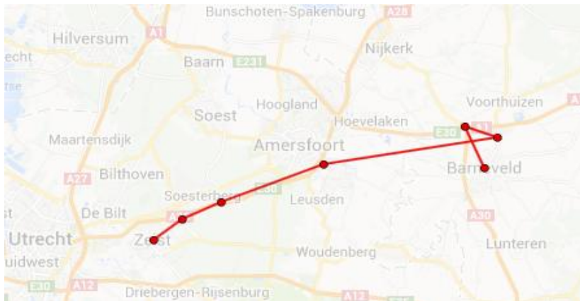
Figure 5-6: Edges of the shortest path between Zeist and Barneveld (Google).
