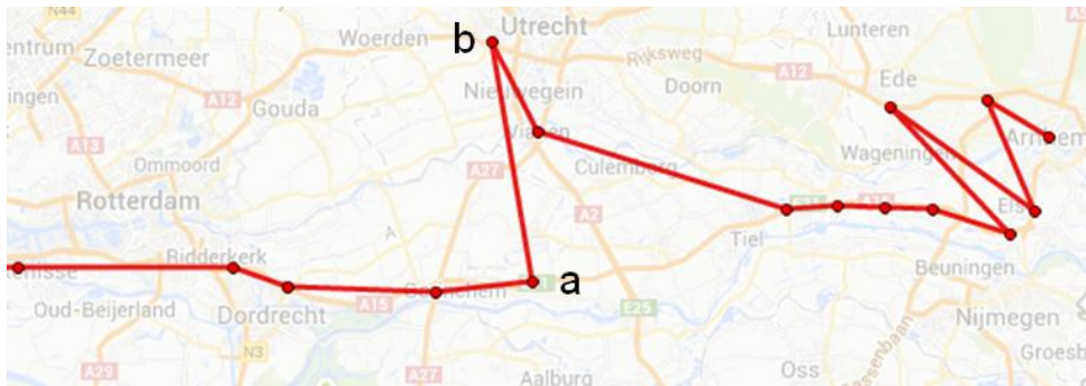
Figure 5-7: Edges determined by our shortest path computations from Hellevoetsluis to Arnhem (Google).
