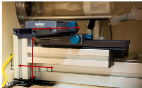
Figure 4.20: A sketch of the degrees of freedom of the camera and camera mount.
