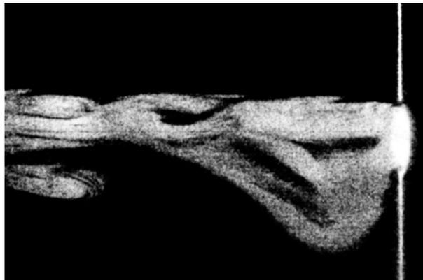
Figure 8.3: Flow visualization at with shutter speed 1/1000 sec, F/3.2 and ISO 25,600 with tube open
