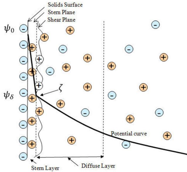
**Figure 11:** Schematic of the electric double layer on membrane surface according to stern model consisting of an immobile stern layer and a diffusion region. [41]
