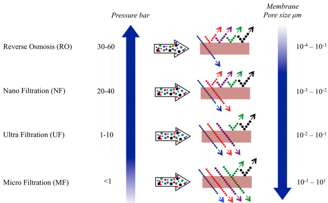
**Figure 1:** Schematic overview of membrane separation processes: reverse osmosis (RO), nanofiltration (NF), ultrafiltration (UF), microfiltration (MF) and the corresponding properties such as pressure, separated ions and pore sizes. [12]
