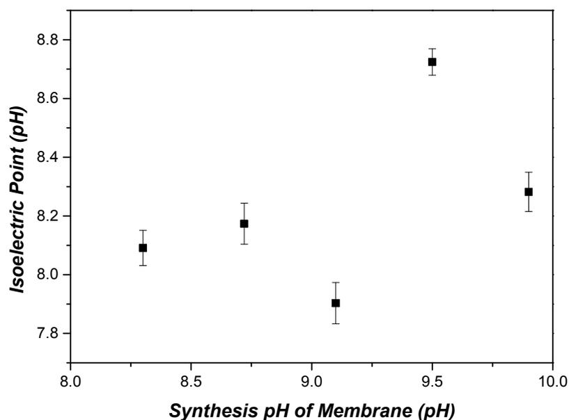
**Figure 23:** Isoelectric points for IDC POSS membranes as a function of synthesis pH value of IDC POSS membranes.
