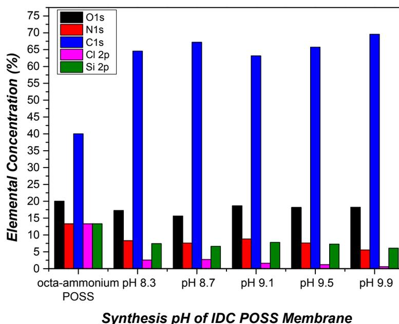
**Figure 16:** Elemental concentrations of octa-ammonium POSS and IDC POSS membranes synthesized at various pH values (pH 8.3, 8.7, 9.1, 9.5, 9.9). Different bars depict the oxygen (O1s –), nitrogen (N1s –), carbon (C1s –), chloride (Cl2p –) and silicon concentration (Si2p –).
