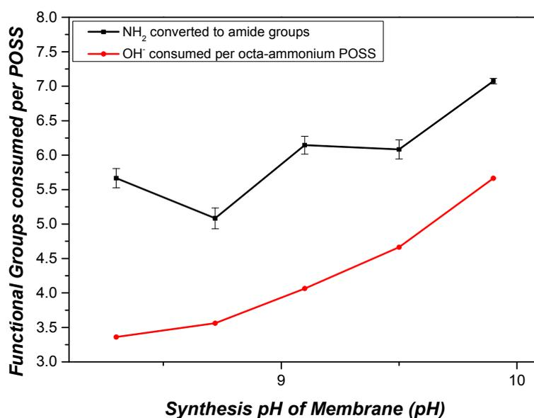
**Figure 19:** Functional groups consumed per POSS cage in reaction as a function of synthesis pH of IDC POSS membranes. The red line is the number of hydroxyl ions ( $\text{OH}^-$ ) consumed per octa-ammonium POSS molecule while the black line shows number of primary amine groups converted to amide groups per POSS molecule. The error bars in the black line are based on standard errors in peak fitting.
