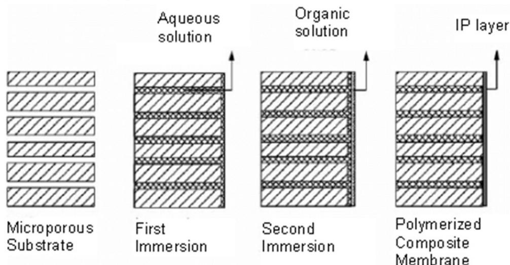
**Figure 2:** Schematic overview of TFC membrane synthesis steps via interfacial polymerization [18]
