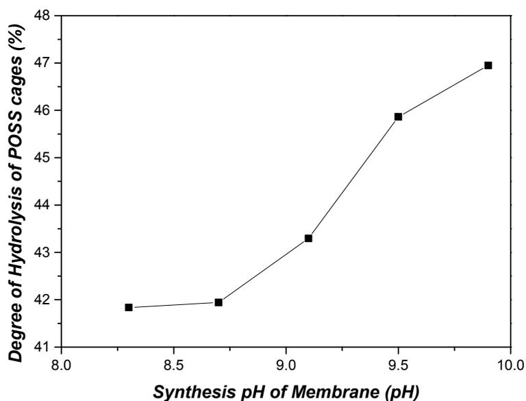
**Figure 15:** Degree of hydrolysis of POSS cages as a function of synthesis pH of IDC POSS membranes. The degree of hydrolysis was calculated by intensity ratios of the ladder and polyhedral POSS peaks.
