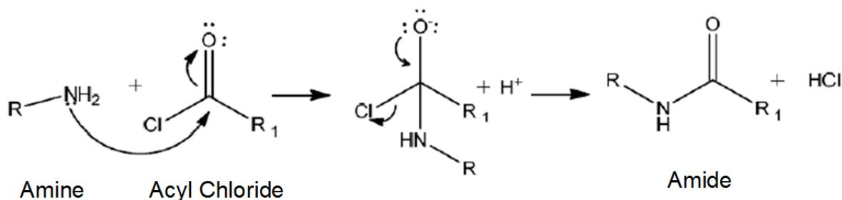
**Figure 3:** Reaction mechanism of an amide via condensation reaction. There is a nucleophilic attack of the amine group to the carbon atom of the acyl chloride, forming an unstable intermediate. Then, the chloride atom leaves as it is a good leaving group and thus an amide bond is formed. The figure exemplifies the polycondensation reaction by the reaction of one functional group. Since multiple functional groups exist, a hyper cross-linked network is synthesized. [20]
