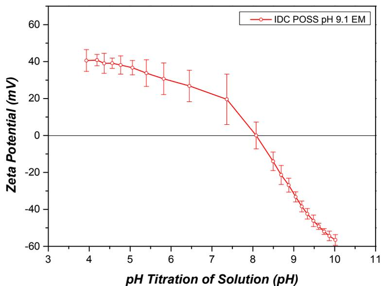
**Figure 29:** Zeta potential for IDC POSS membrane synthesized at pH 9.5 on 7/3/2014 including error bars (95% CI) as a function of pH of the titration solution.
