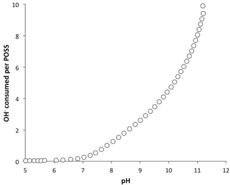
**Figure 6:** Amount of OH<sup>-</sup> consumed per POSS cage as a function of pH of titration solution. [4]
