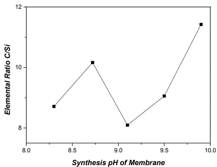
**Figure 28:** Elemental ratio of carbon to silicon as a function of the synthesis pH of IDC POSS membranes.
