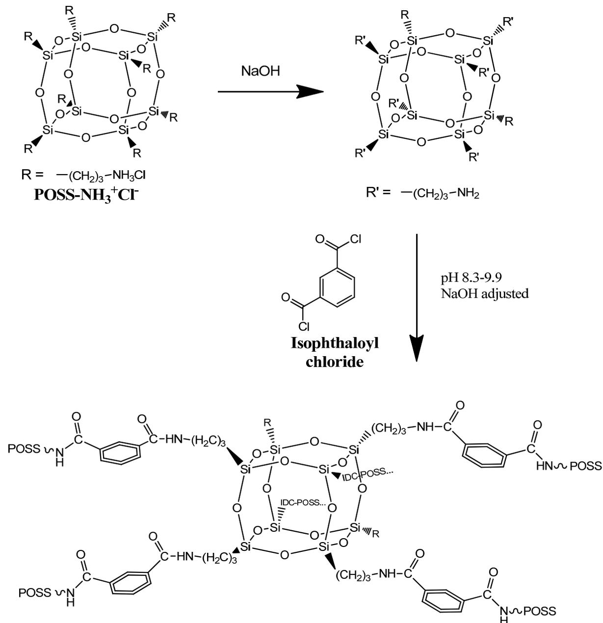
**Figure 24:** Reaction scheme of the interfacial polymerization. In the first step octa-ammonium groups of POSS cages are partially deprotonated, resulting in reactive primary amine groups. The amine groups react in a polycondensation reaction with IDC through which the subsequent network is formed.
