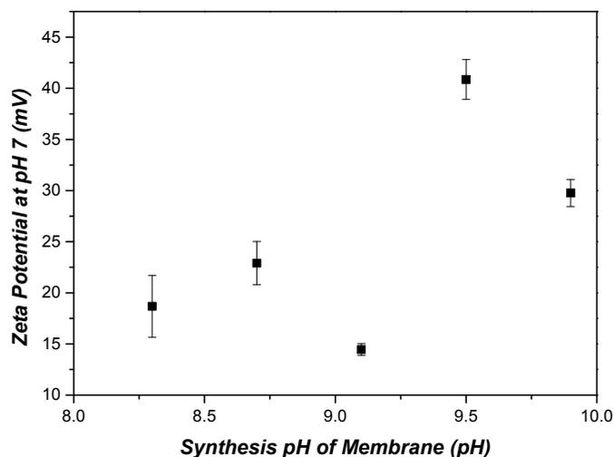
**Figure 30:** Zeta potential in neutral solution environment (pH 7) as a function of the synthesis pH of the IDC POSS membranes.
