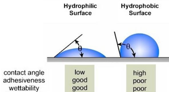
Figure 12: Overview of hydrophilic and hydrophobic surfaces with corresponding characteristics of contact angle, adhesiveness and wettability.[46]
