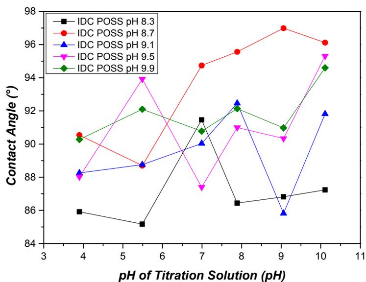
**Figure 31:** Contact angle pH titration for IDC POSS membranes synthesized at different pH values (pH 8.3 – 8.7 – , 9.1 – , 9.5 – , 9.9 –) as a function of the pH of the different titration solutions.
