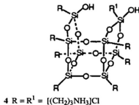
**Figure 7:** Ladder structure of octa-ammonium POSS cage. [24]
