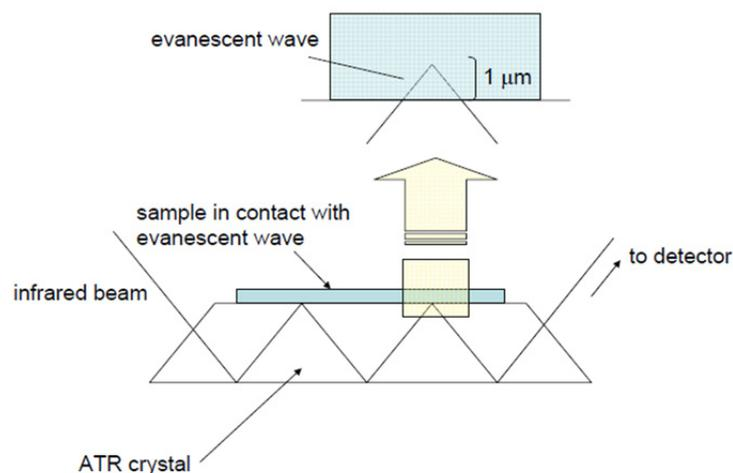
**Figure 9:** Schematic view of attenuated total reflection infrared spectroscopy. The incoming IR beam is multiple times reflected between sample surface and ATR crystal before it is detected and an interferogram is obtained. [35]
