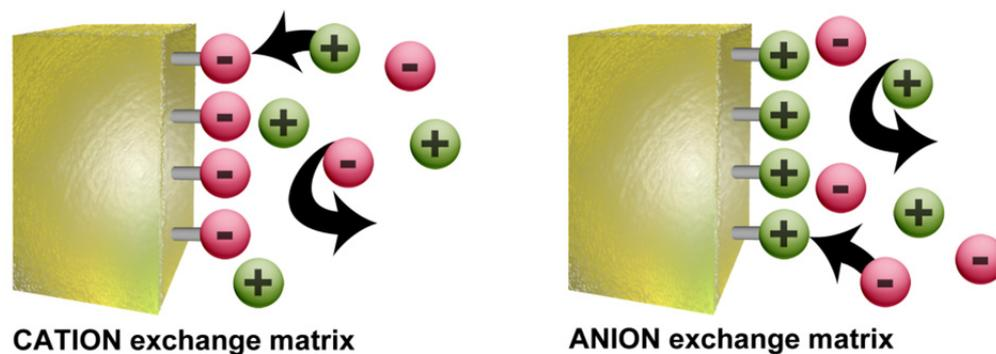
**Figure 8:** Schematic of the Donnan-exclusion effect for positively charged membranes (anion exchange matrix) and negatively charged membranes (cation exchange matrix) [27].
