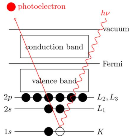
**Figure 10:** Principle of X-ray photoelectron spectroscopy. The X-ray energy ( $h\nu$ ) excites and emits a photoelectron with a certain kinetic energy. K, L<sub>1</sub> and 1s, 2s, 2p label the shells or orbital, respectively. [39]
