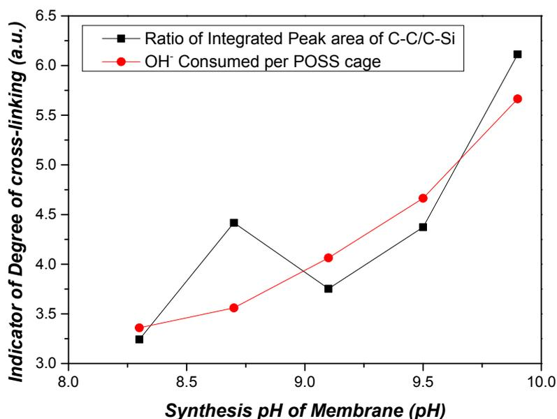
**Figure 21:** Indicator of degree of cross-linking as a function of synthesis pH of IDC POSS membranes. The red line is refers to the OH<sup>-</sup> consumed per POSS cage as a function of preparation pH of the membrane (reference) expected. The black line shows the ratio of integrated peak area of C-C and C-Si of the experimental XPS data as a function of the synthesis pH of the IDC POSS membranes.
