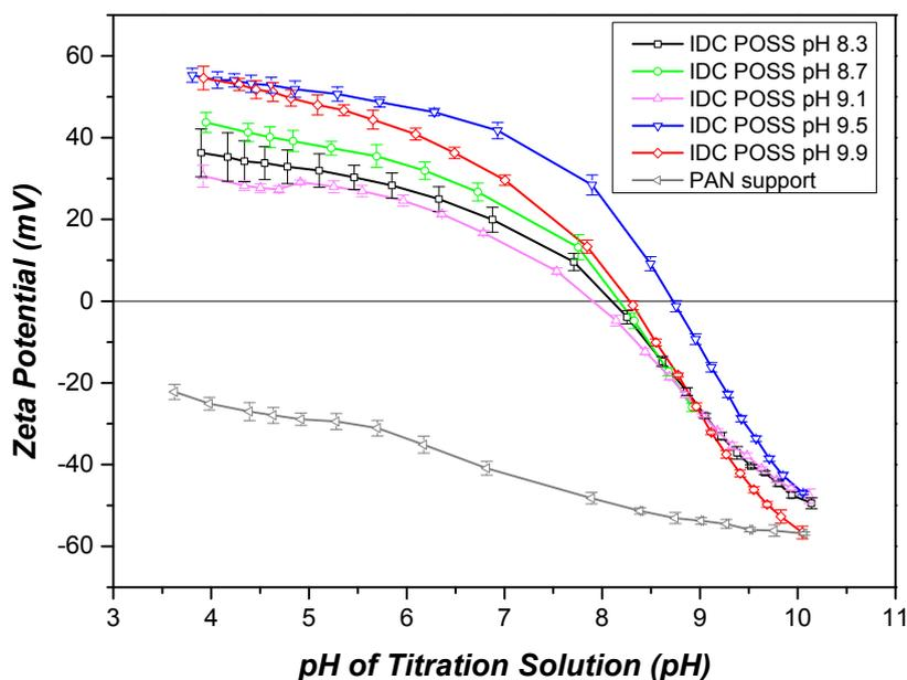
**Figure 22:** Zeta potential as a function of pH of titration solution for IDC POSS membranes synthesized at different pHs (pH 8.3 –, 8.7 –, 9.1 –, 9.5 –, 9.9 –) and the PAN support (–) as reference spectrum. The error bars show the 95% confidence interval.
