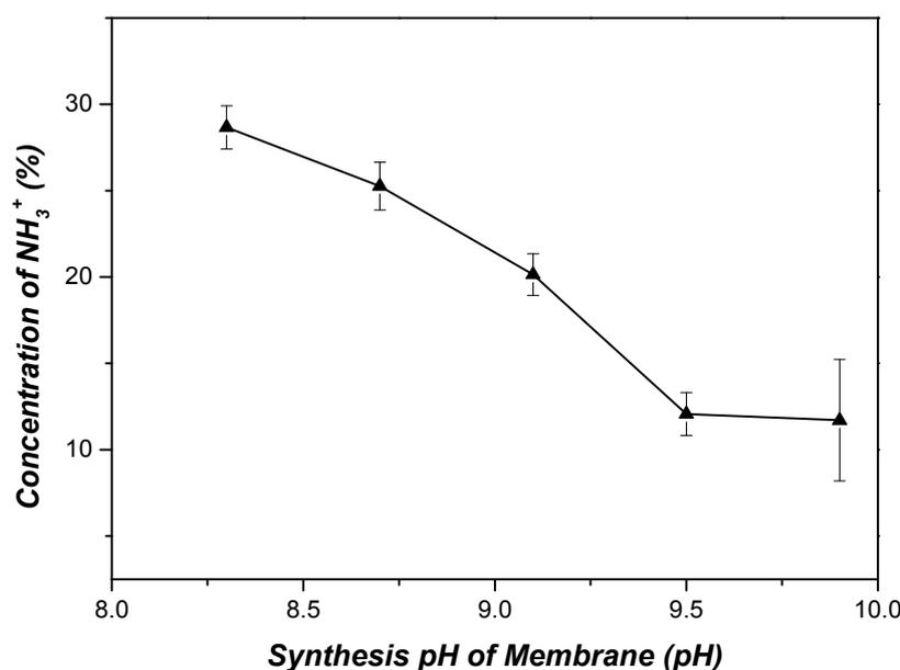
**Figure 18:** Concentration of ammonia groups as a function of the synthesis pH of IDC POSS membranes. The error bars indicate the standard error in the peak fitting.
