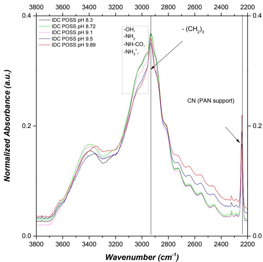
**Figure 25:** Normalized infrared absorbance spectra (zoom of 3800-2200  $\text{cm}^{-1}$ ) of IDC POSS synthesized at different pH values (pH 8.3 —, 8.7 —, 9.1 —, 9.5 —, 9.9 —)
