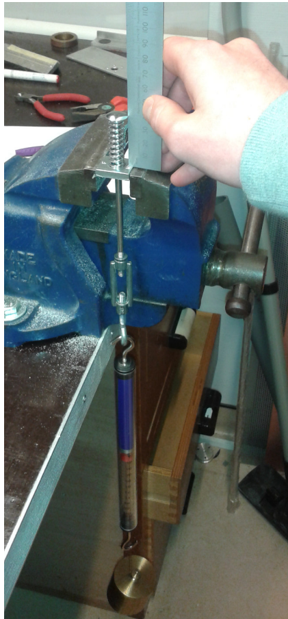
Figure A.9: Setup for the measurement of the Spring constant k including Newton-meter, weights(below) and scale.
