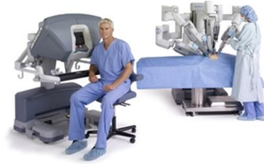
Figure 4 Da Vinci System (console and robotic arms)
