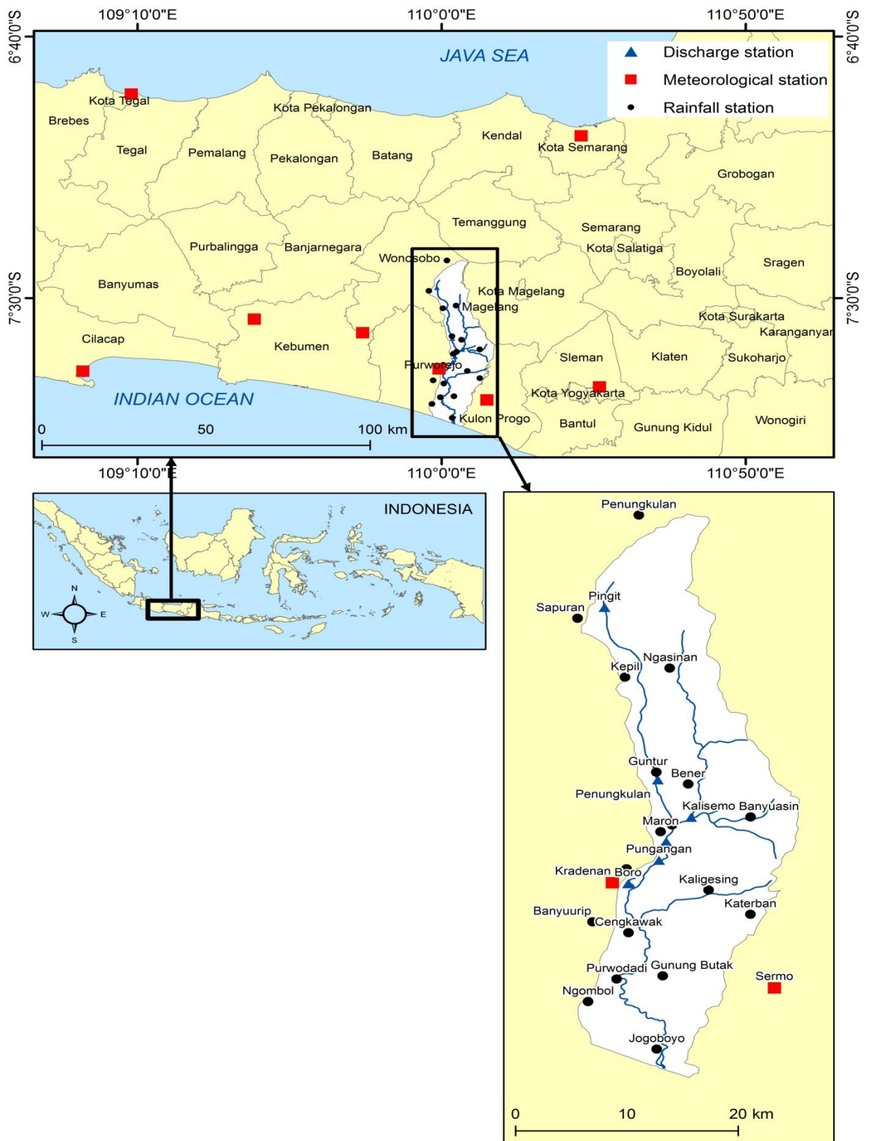
Figure 2.1: Location of Bogowonto catchment and position of river & distribution of hydro-meteorological gauges (Marhaento, 2014). Black = rainfall stations, red=meteorological station, blue=discharge station.
