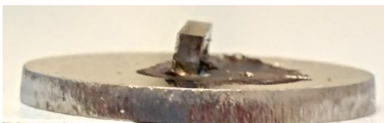
Figure 27. Image of the sample plate and the sample on top, slightly skewed by the amount of silver paste, of which the excess can be seen around the sample.
