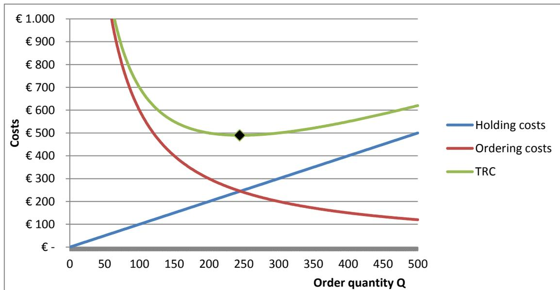
Figure 4.1 - The Total Relevant Cost function (convex function)
