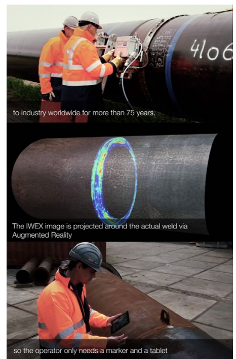
Figure 1.30: Applus+ RTD iPad application by TWNKLS to inspect weld
