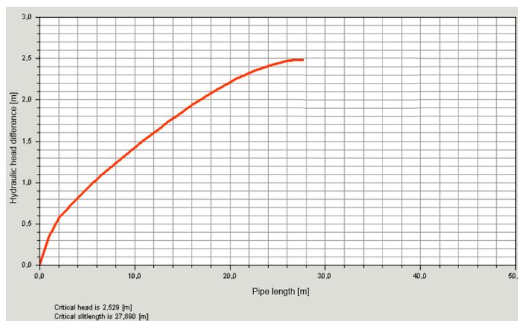
**Figure 2-2 Example of the Sellmeijer model (Mseep) output: the equilibrium curve with  $\Delta H_{CRIT}$  (2.53 m) and critical pipe length (28 m). The total seepage length is 40 meters**
