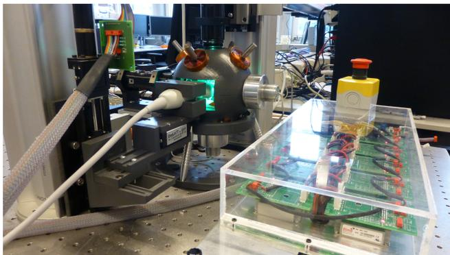
Fig. 20. Photograph of the new setup, which was realized by 3D printing parts from CAD drawings, adding a layer of paint and attaching parts together with bolts.
