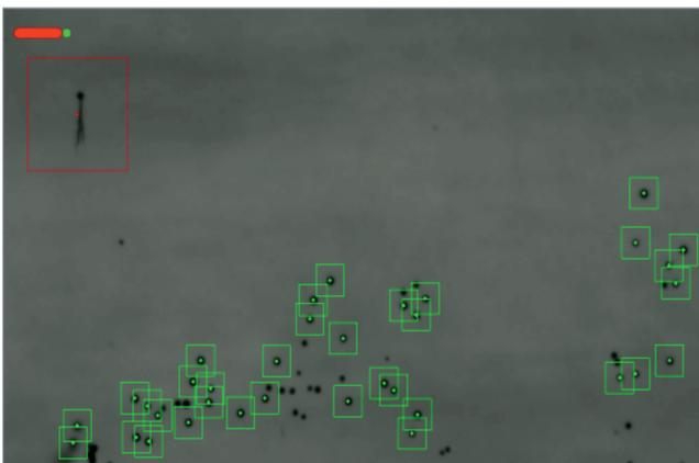
Fig. 25. Multi-agent tracking applied to bubbles using the microparticle tracker settings and a microjet using the microjet tracker settings.
