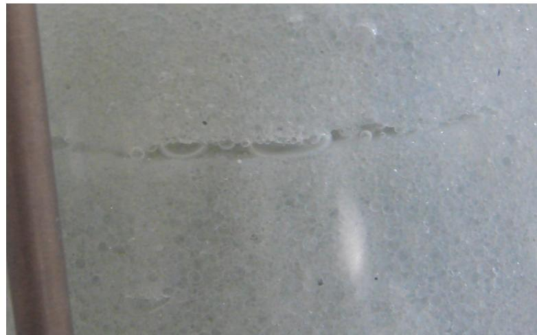
FIGURE 6.3: Crack developed in non-uniform sample
