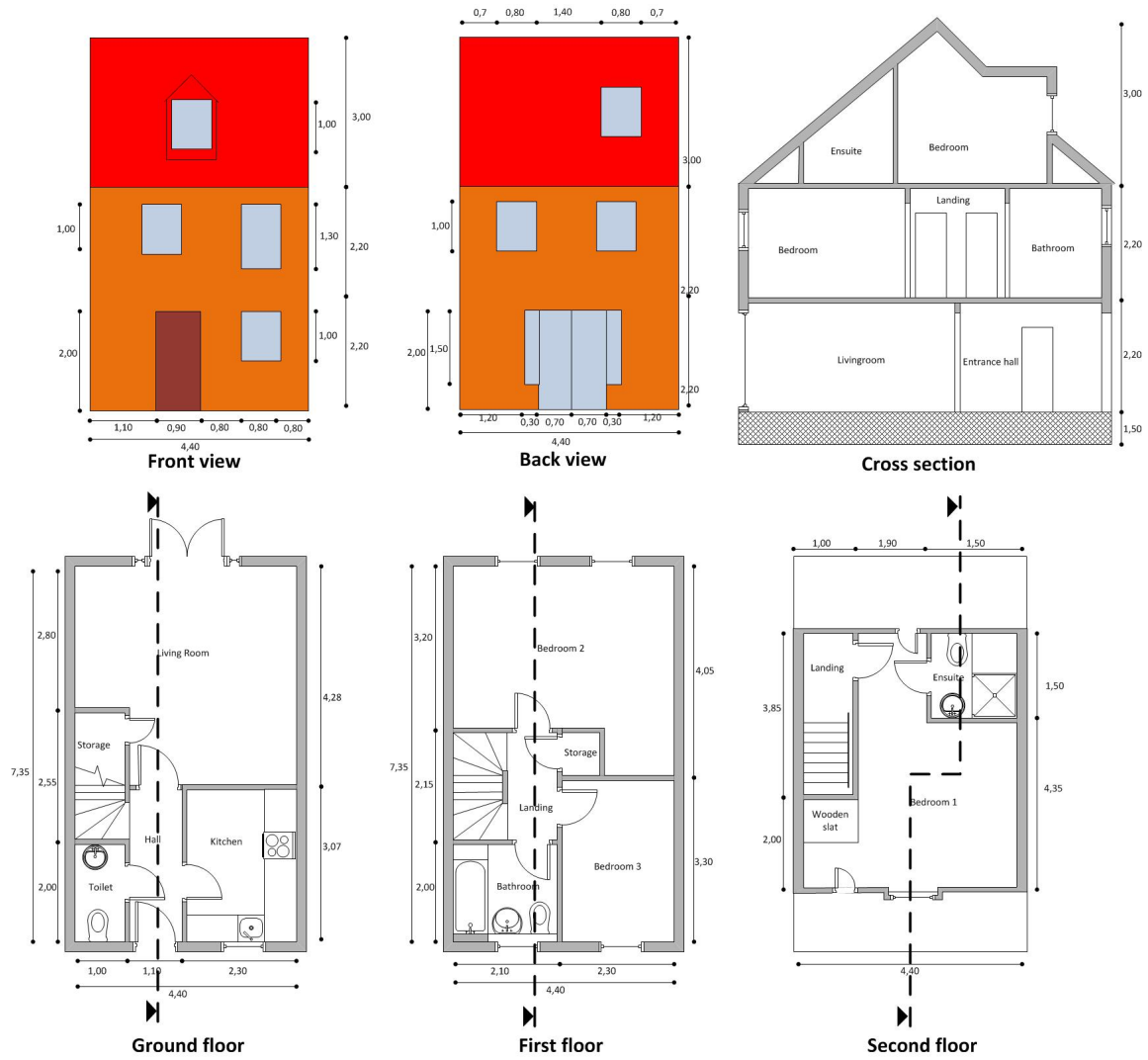
Figure 3.2: Technical drawings of commonly terraced house with dimensions in m
