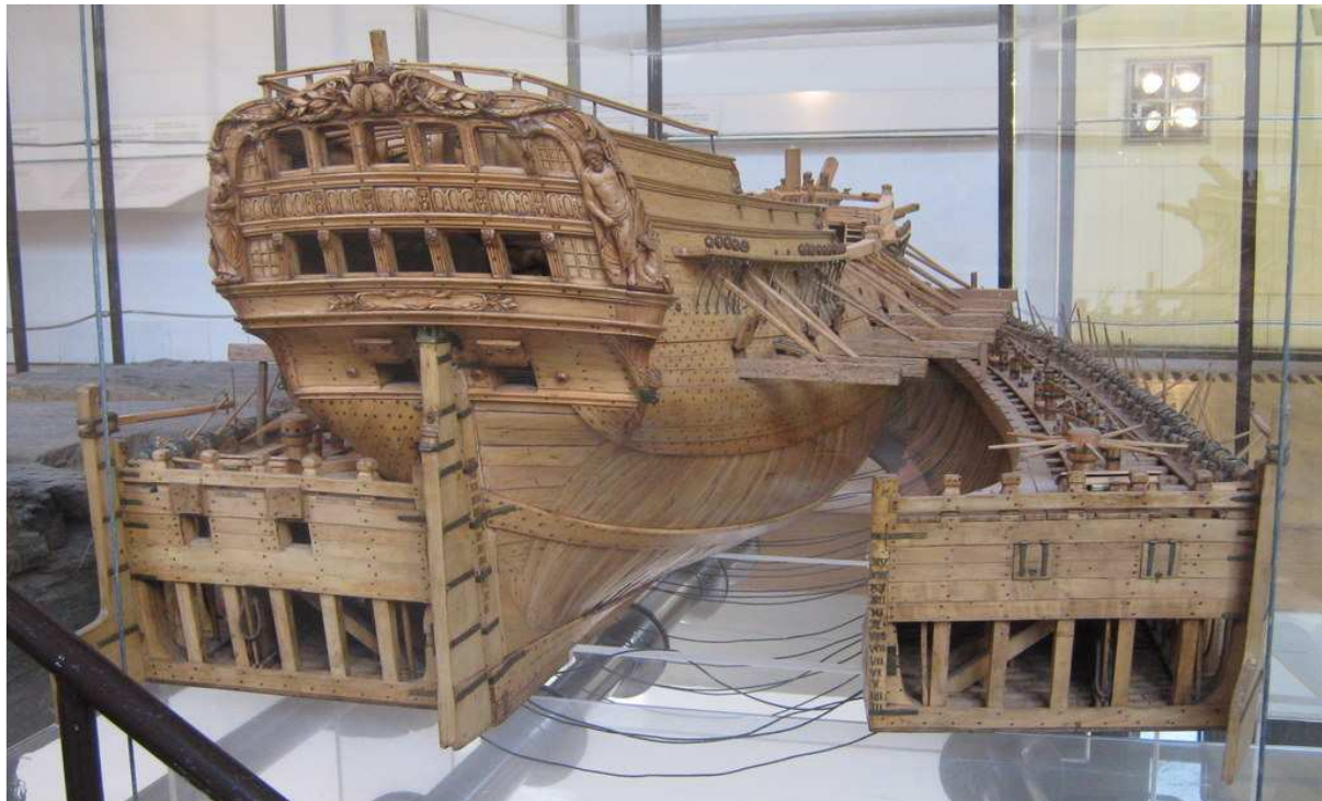
Fig. 3.4 Model of a 150ft. retourschip in “camels” 324 , made by Charles Bentam in the 1740s; currently in the collection of the Amsterdam Historisch Museum. Photo taken by Johan de Jong on 11 Feb 2010
