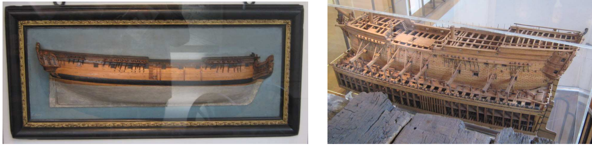
Fig. 5.1 Halfmodel of a naval frigate (left) and full model of a 150 ft. VOC retourschip (right), both currently in the collection of the Amsterdam Historisch Museum. These models were made by the English master shipwright Charles Bentam. Photo taken by Johan de Jong on 11 Feb 2010
