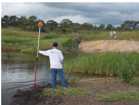
Figure 17 Total station measurement
