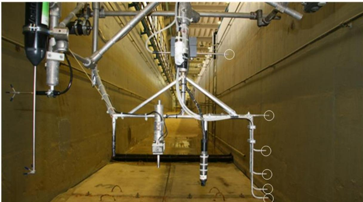
Figure 4: Measuring frame with the suction nozzles on the right side (original photo by Van Der A)
