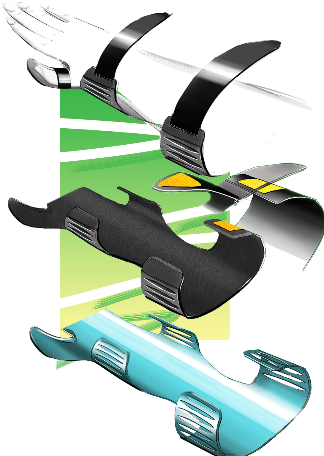
Figure 68. End proposal: Plastic model, black padding and location of the straps
