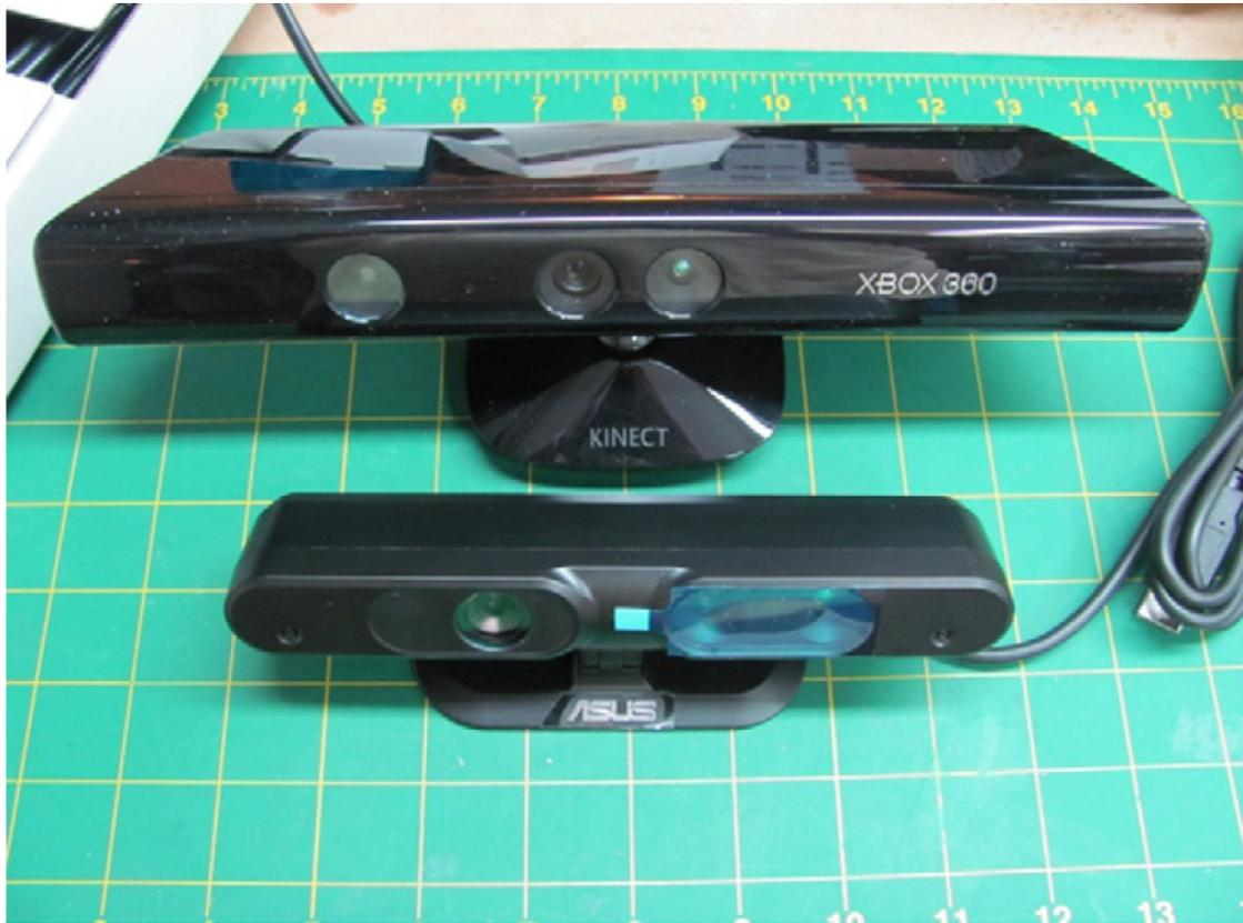
Figure 13: Size comparison between the Microsoft Kinect and the Asus Xtion [37]
